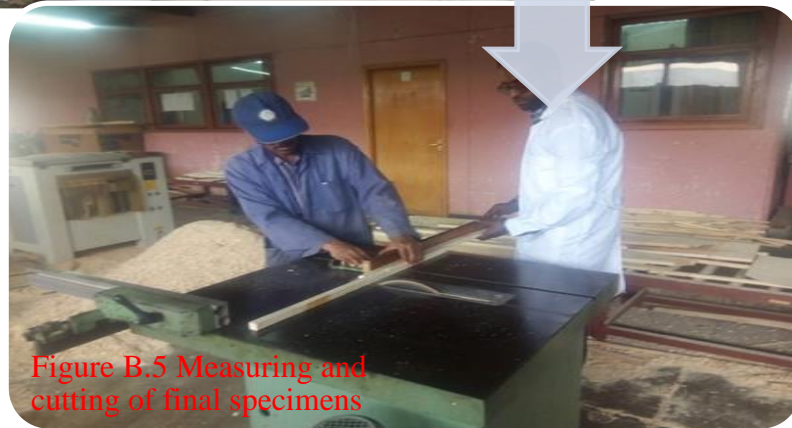
Figure B.4 Reducing the size of battens
