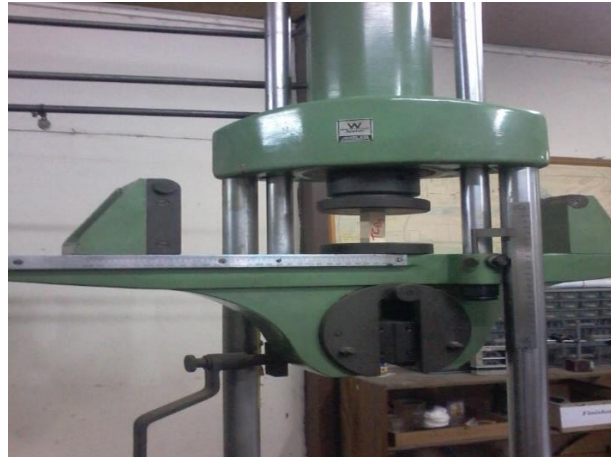
Figure 3-2: Test set up for Compression parallel to the grain test
