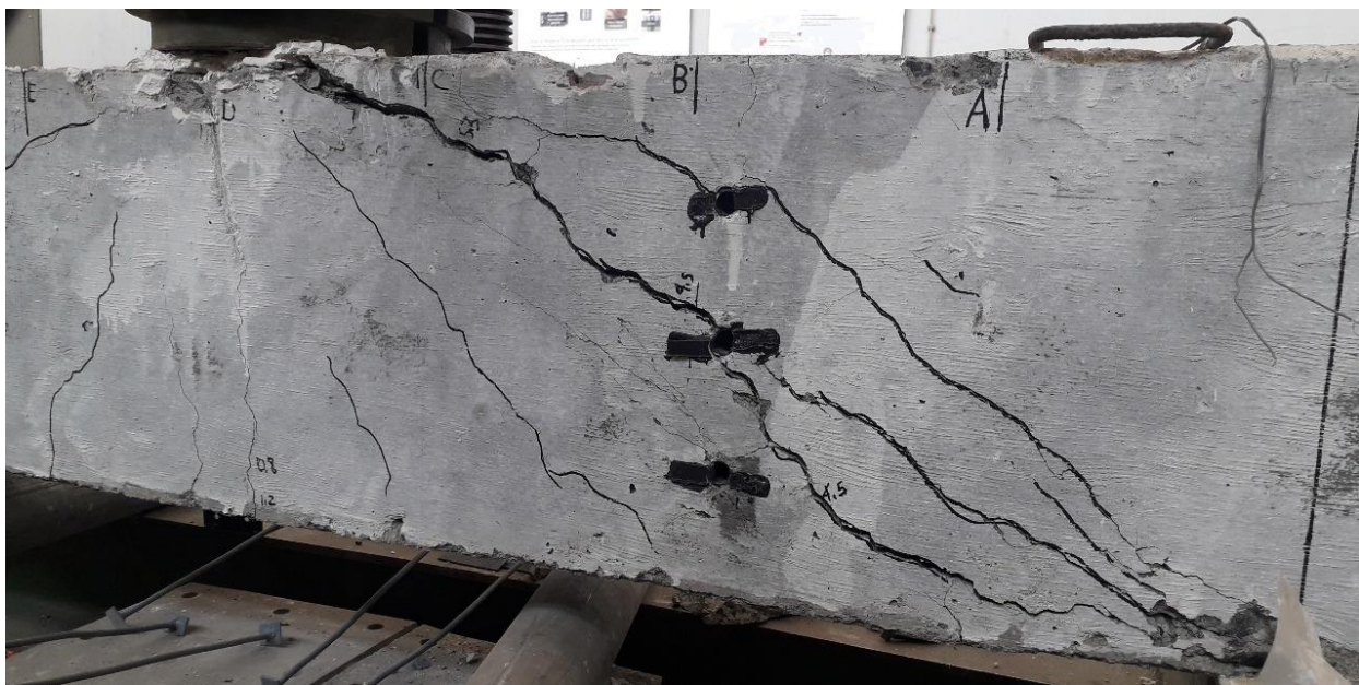
Figure 4-13: Back Side Diagonal Compression Cracks at Failure (SI8-25)
