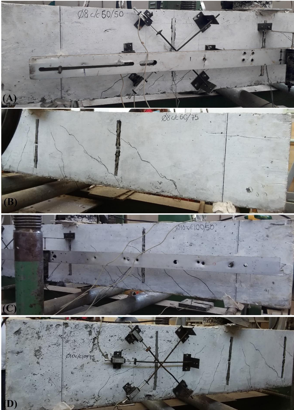
Figure 4-2: Trial Specimen After the First 9 Cycles of Loading (A.TR 8-50 / B.TR 8-75 / C.TR 10-50 / D.TR 10-75)
