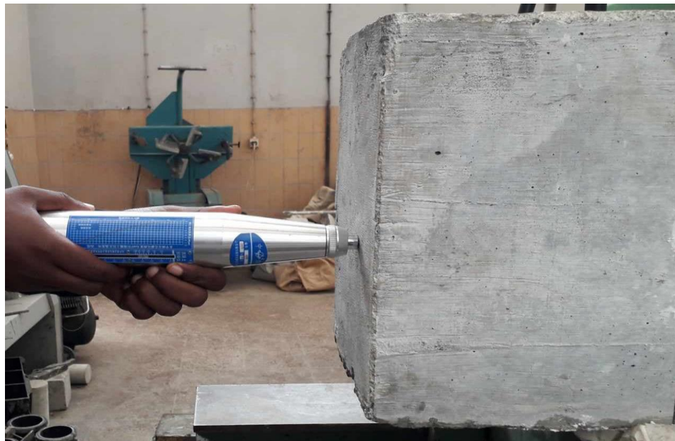
Figure 3-31: Rebound/ Schmidt Hammer Test
