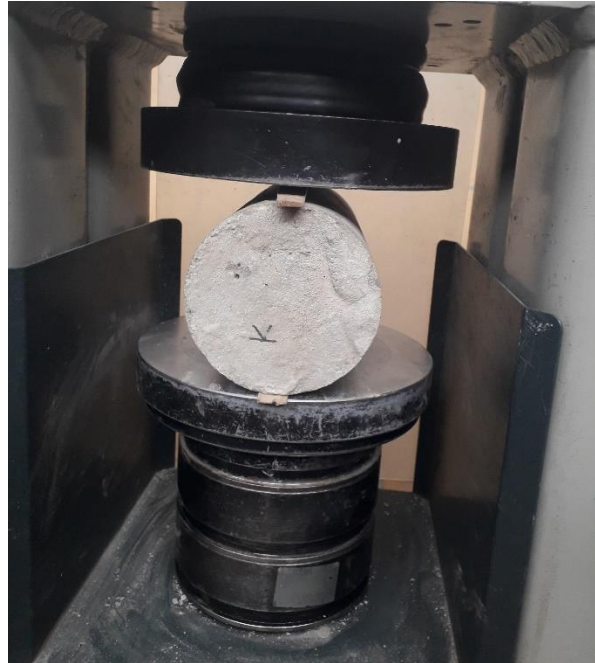
Figure 3-8: Split Cylinder Test for Tensile Strength
