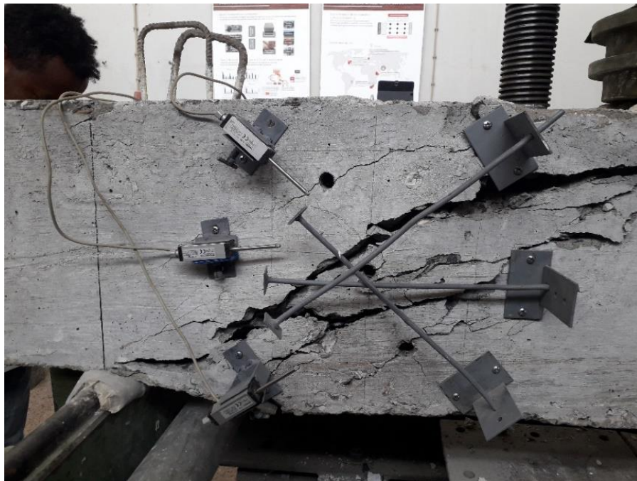
Figure 6-19: Out of Plane Deformation Disrupting Surface Displacement Measurements
