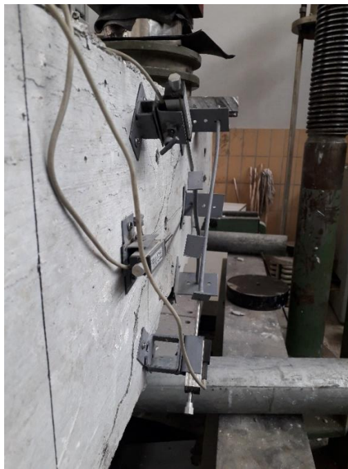
Figure 4-19: Misalignment of Surface Measurements due to Out of Plane Deformation II (SI8-50)
