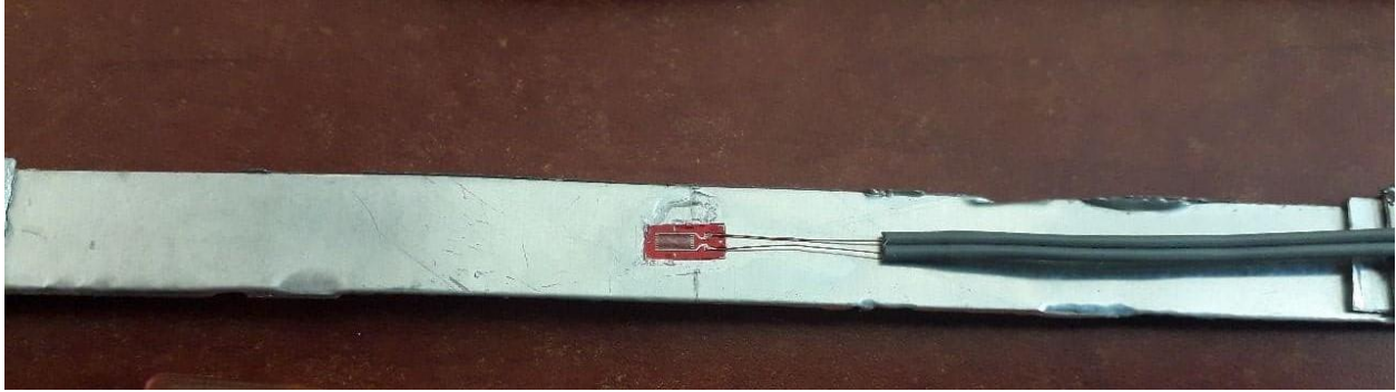
Figure 3-35: Strain Gauge Attached in the Middle of Aluminum Strip
