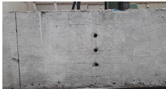
Figure 6-13: Modified Out of Plane Instrumentation Holes for Main Specimens
