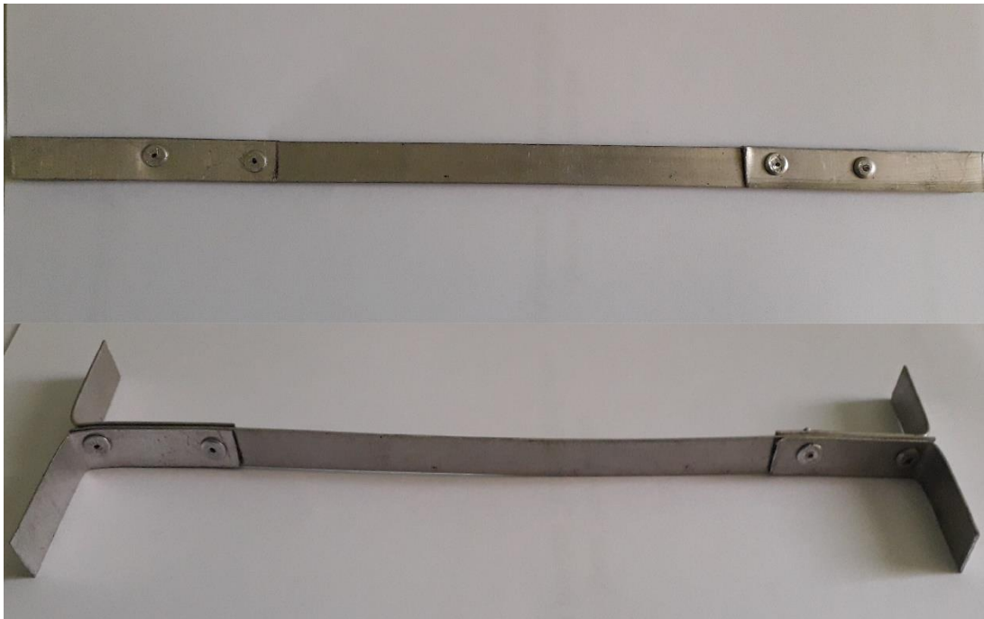
Figure 3-34: Aluminum Strips used for Out of Plane Strain Measurement
