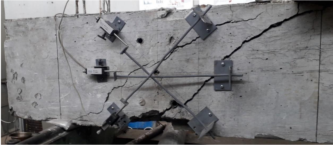
Figure 4-18: Misalignment of Surface Measurements due to Out of Plane Deformation I (SI8-50)
