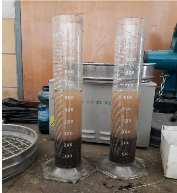
Figure 3-6: Silt Content Test for Fine Aggregate
