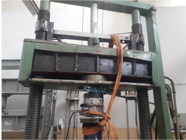
Figure 3-24: Reaction Frame After Stiffening Modification
