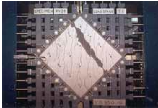
Figure 2-2: 1986, Vecchio FJ and Collins MP. Modified Compression Field Theory, Membrane Element Test
