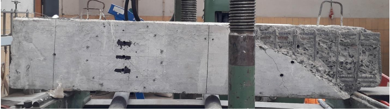
Figure 4-35: Final State of the Beam (SIII10-75)
