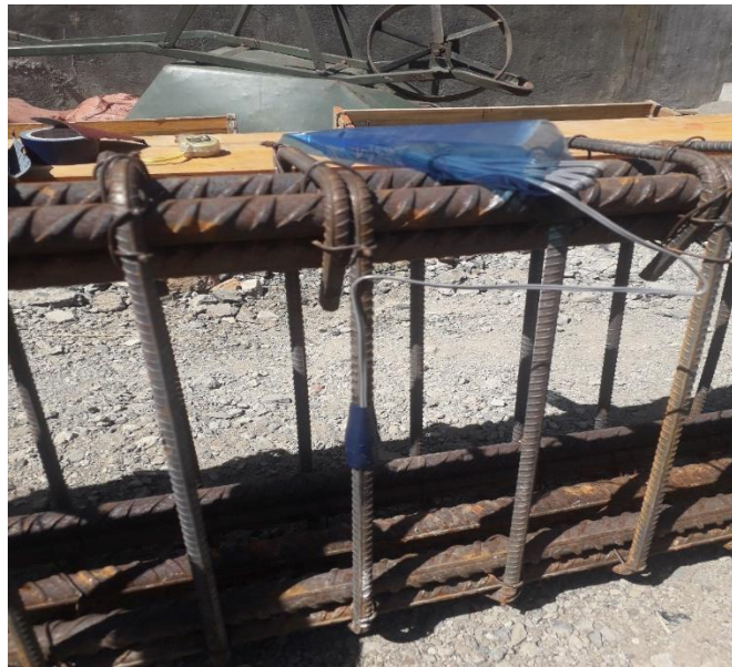
Figure 3-15: Strain Gauge Placement on Stirrup
