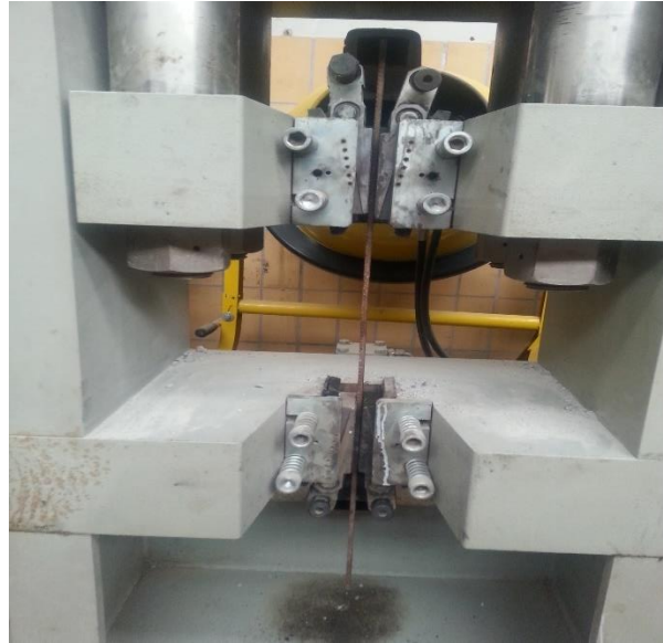
Figure 3-9: Uniaxial Tensile Test on Reinforcement
