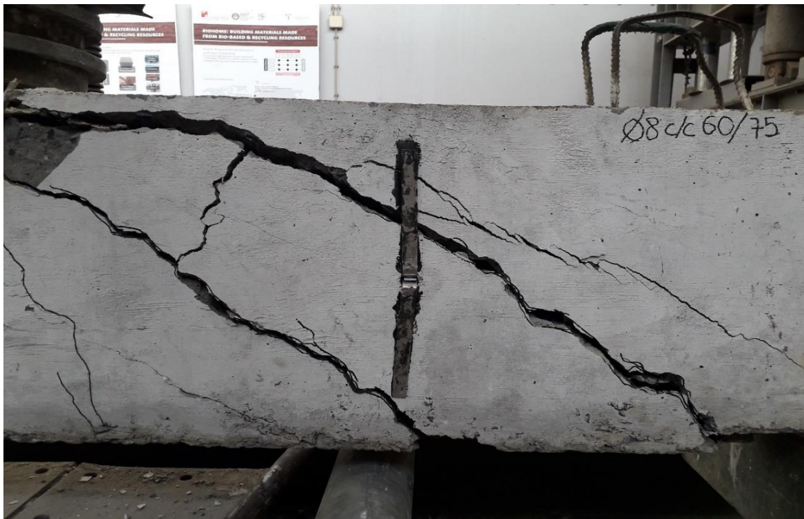
Figure 4-5: Diagonal Shear Cracks at Failure, 75mm Side Cover (TRIAL Beam (TR 8-75))
