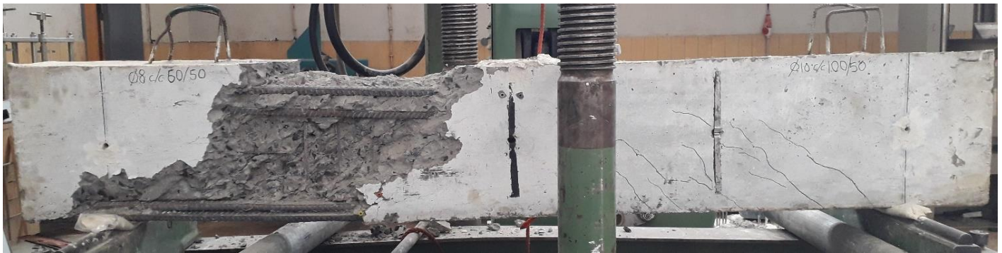
Figure 4-9: Final State of Beam After Failure (TRIAL Beam)
