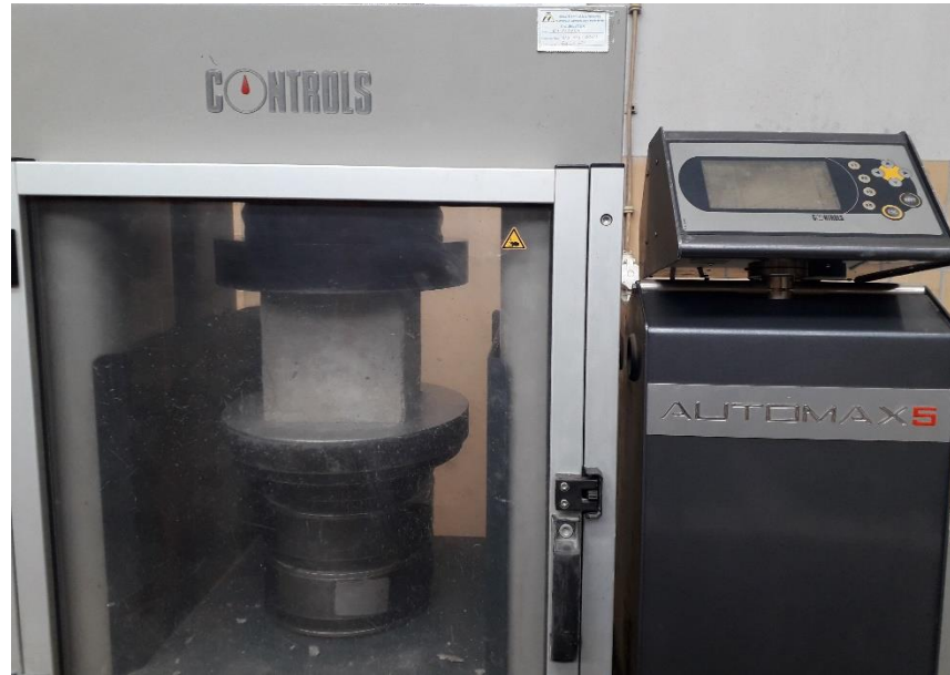
Figure 3-7: Concrete Compressive Test on Cube
