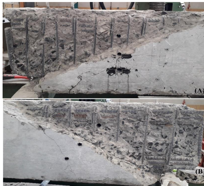
Figure 6-27: Spalled Section Roughness Variation (A) SIII8-75 (B) SIII10-75
