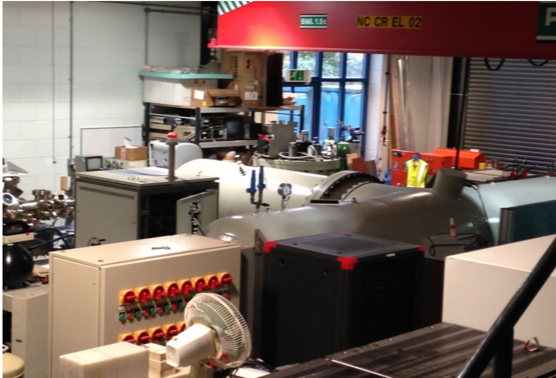
Figure 4-5 The High Voltage Engineering Europe 2.0 MV Medium Current Plus Tandron™ accelerator providing 2.5 MeV protons. The facility is situated in the Surrey Ion Beam Centre.
