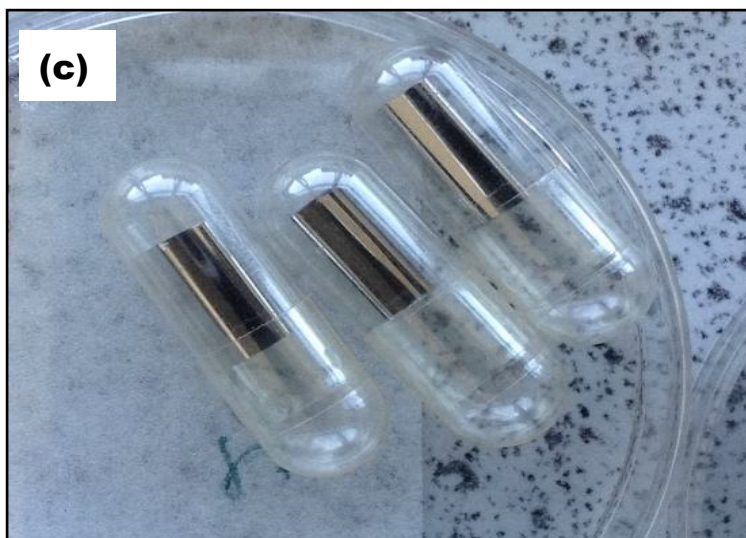
Figure 5-7 Equipment used for sample preparation of TL dosimetric system studied; (a) vacuum tweezers, (b) balance, (c) gelatine capsules.
