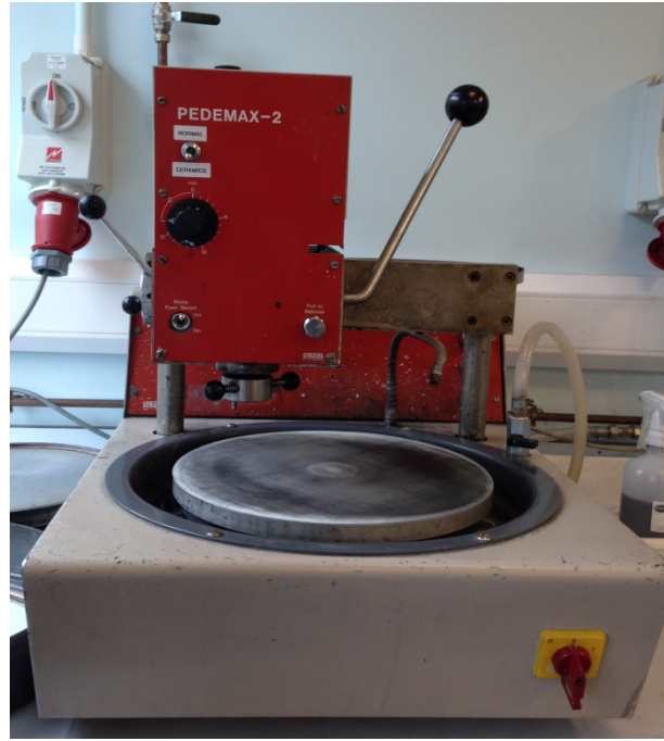
Figure 4-3 Pedemax-2 was employed for sample preparations. The rotating circular lapping machine is featured in this photograph; a disc of fine abrasive medium is attached to the lapping surface such that with even pressure a polished flat surface to the sample assembly can be achieved.
