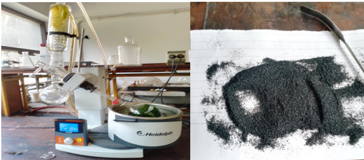
Figure 11: The solvent was removed by rotary evaporator and the dried extract sample
