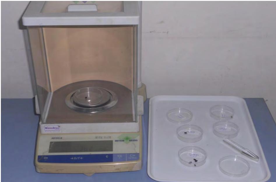
Figure 12. Electrical sensitive balance used for weighing pupae of G.pallidipes at Kality tsetse fly rearing and irradiation center.
