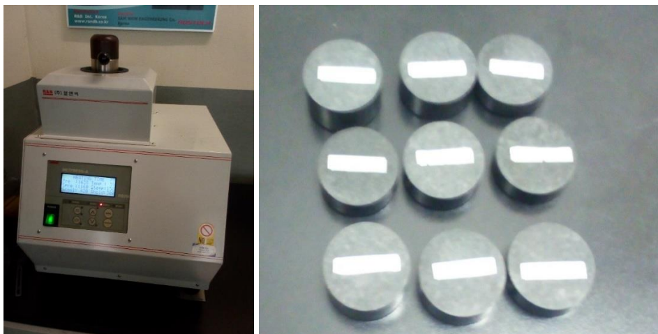
Figure 3. 16 a) Hot mounting press(RB 206 Metpress-A) b) Samples of mounted specimen
