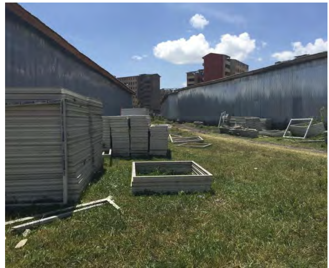
→ PVC window frames scattered on grass for weather effects.
