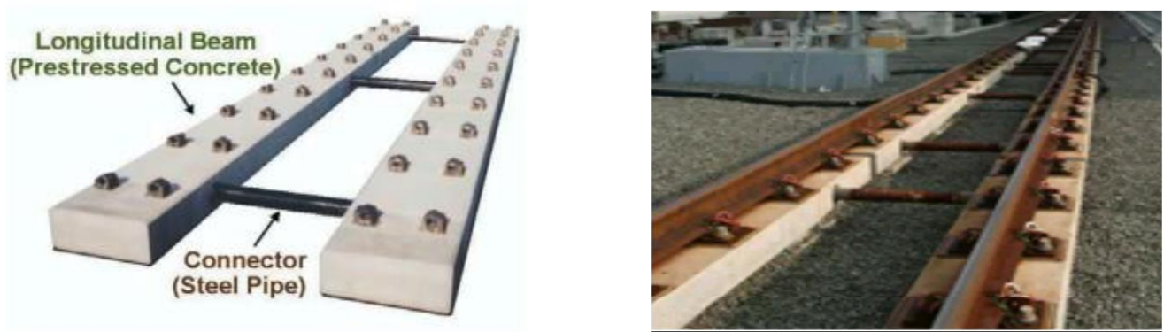
Figure 1.1 3D view of typical ladder track
