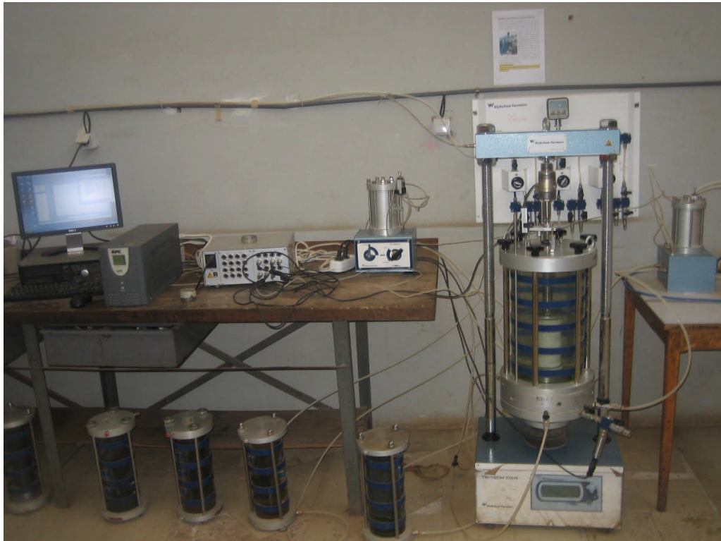
Figure 3-4 Modified triaxial apparatus
