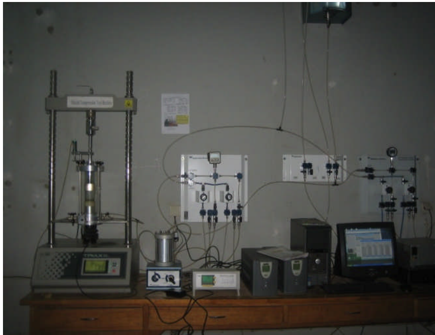
Figure B-3 Conventional triaxial machine used for testing saturated samples
