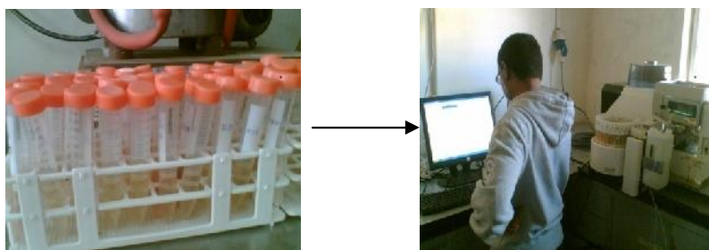
Fig. 7 Detection of the elements (Ca, Fe and Zn) using SHIMADZU AA6800 at EPHI
