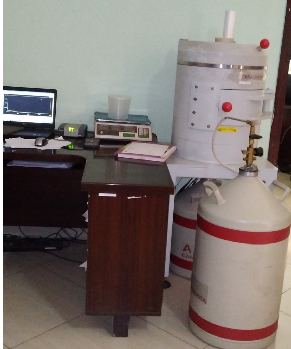
Figure 3.6: Gamma spectrometry mounted with HPGe detector and DSA circuit (ERPA Lab).
