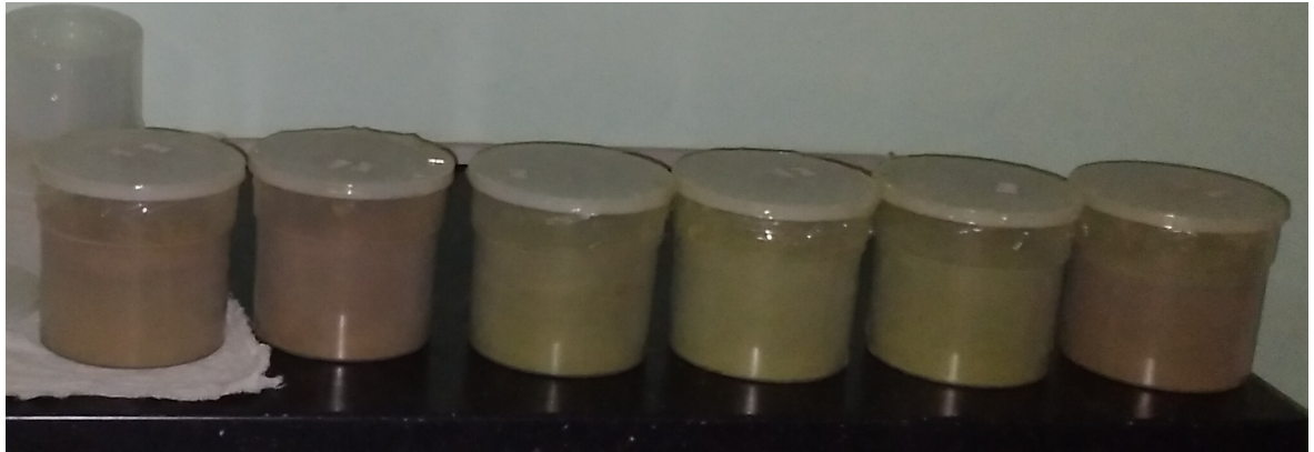
Figure 3.2: Prepared samples of soil and Chat(Khat)for HPGe detector
