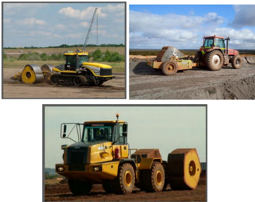
Figure 5: Three, Four and Five Sided Impact Rollers (Sources: M.B. Jaksa and et al [2012] and Landpac)
