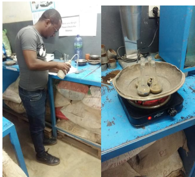
Figure 13: Specific Gravity Test on Progress
