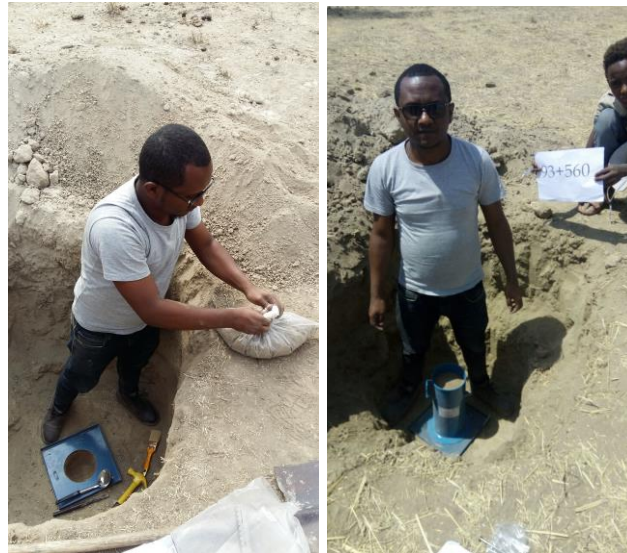
Figure 12: In-Situ Density Determination
