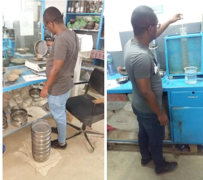
Figure 14: Sieve and Hydrometer Test on Progress
