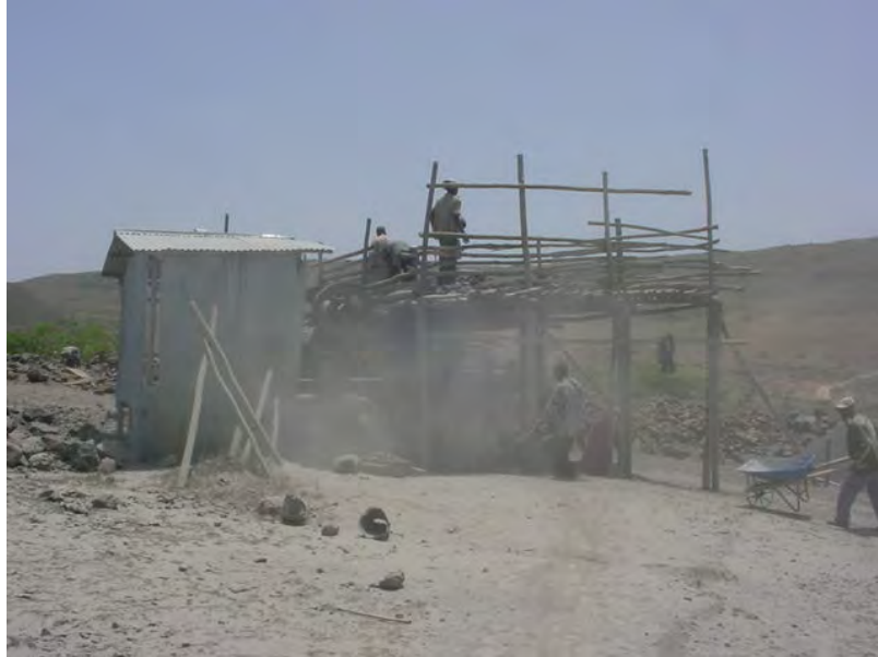
Fig 3.5 Low scaled coarse aggregate crushing plant around Nazreth.
