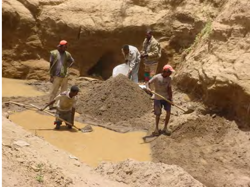
Fig 3.2 Sand being collected from river bed manually around Koka.
