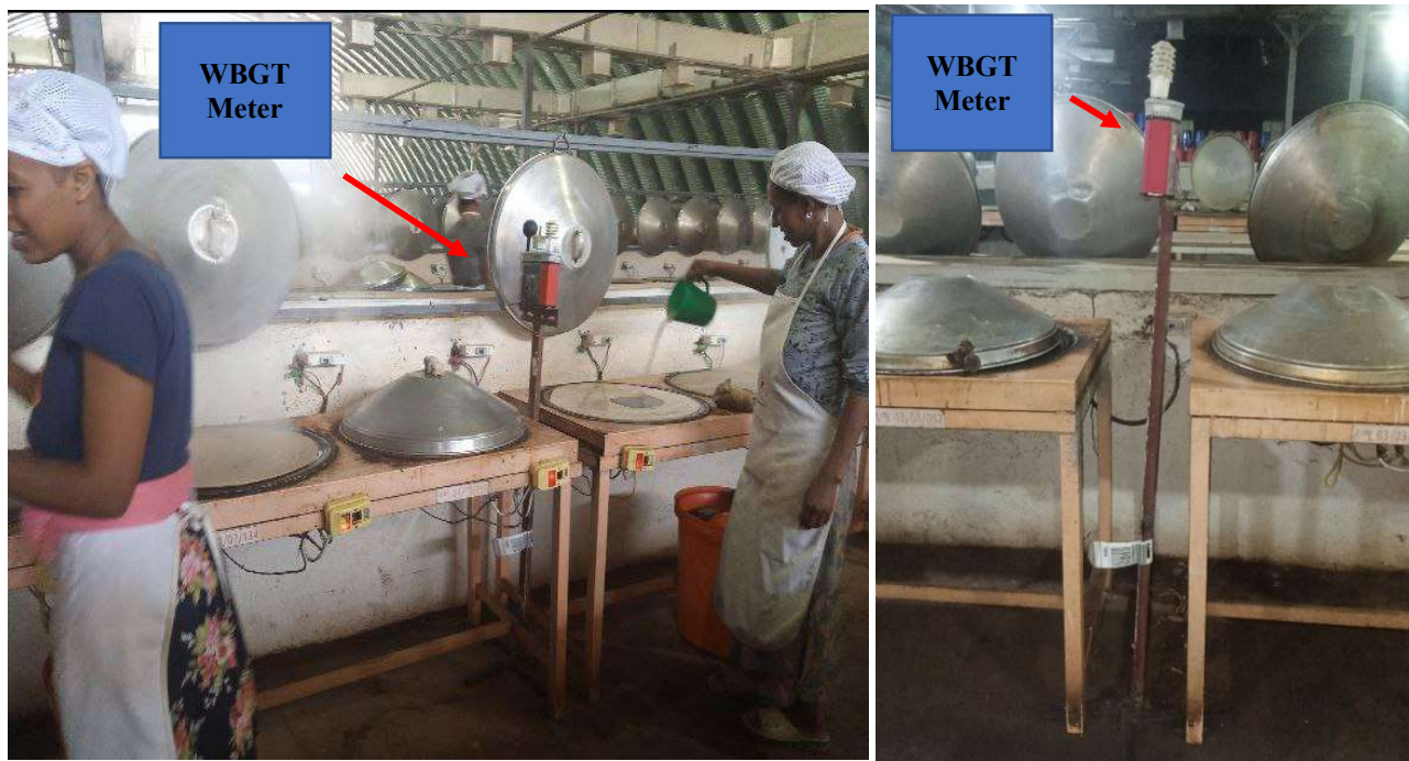
Figure 9: WBGT placement in the Injera Baking area.
