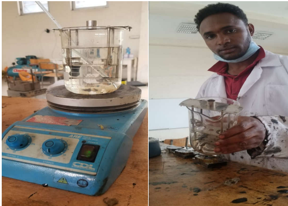
(A) Measuring softening point
