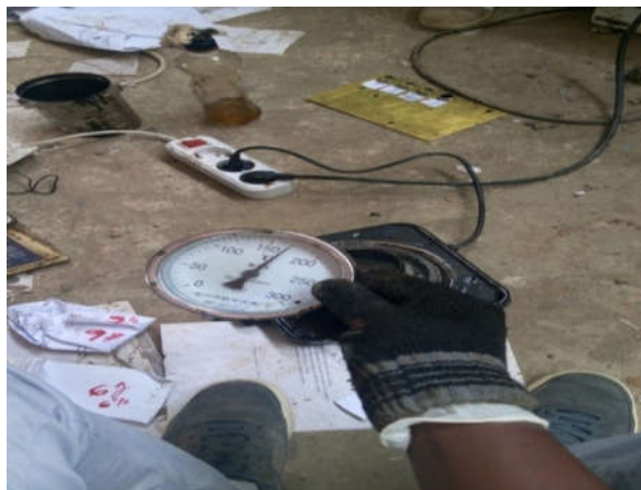
Figure 12: measuring the temperature of the modified bitumen sample
