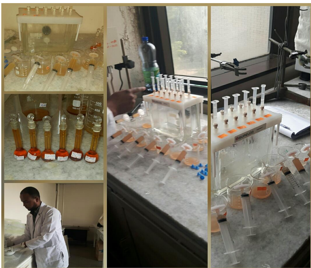
Figure 10: Sample clean-up procedure with immunoaffinity column
