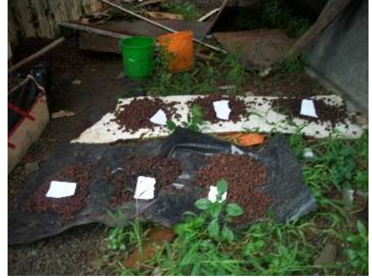
Fig.D6 Soil sample labeling
