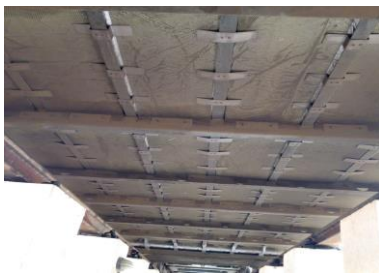
Figure 2.8 AA-LRT vehicles underframe structures
