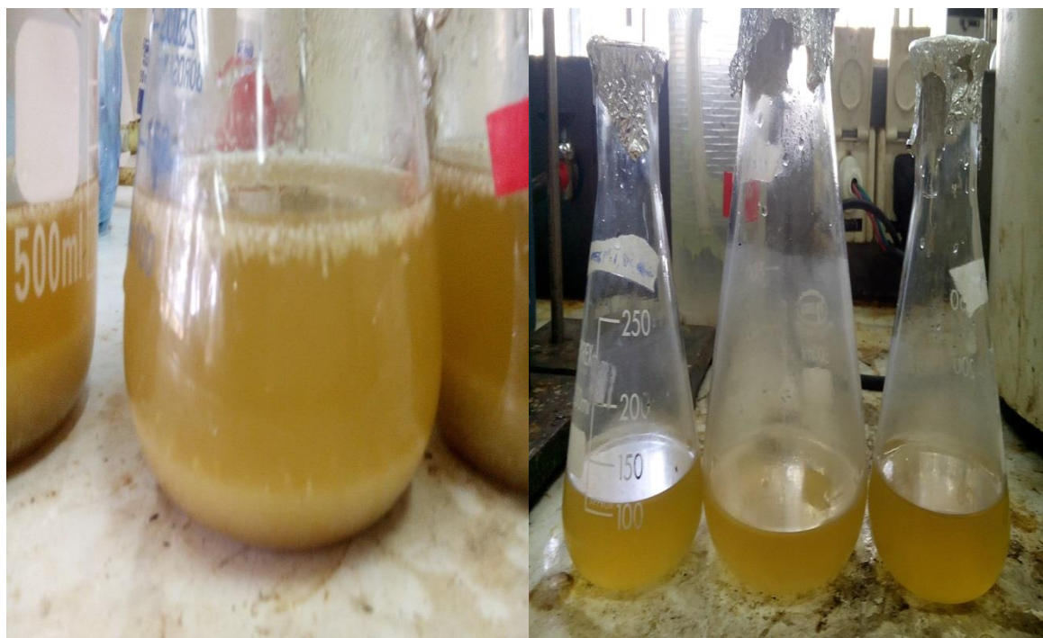
Figure B1-7 At left extraction with residues and at the right clear solution from centrifuge
