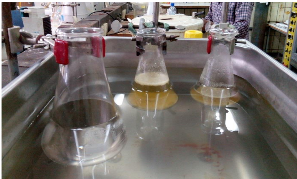
Figure B1-6 Extraction at water bath
