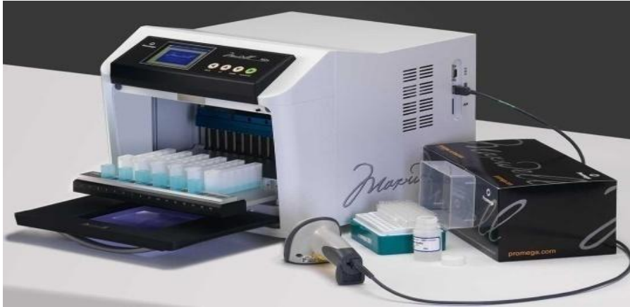
Figure 15 Maxwell® 16 instrument and Levi blood DNA purification kit (Promega)
