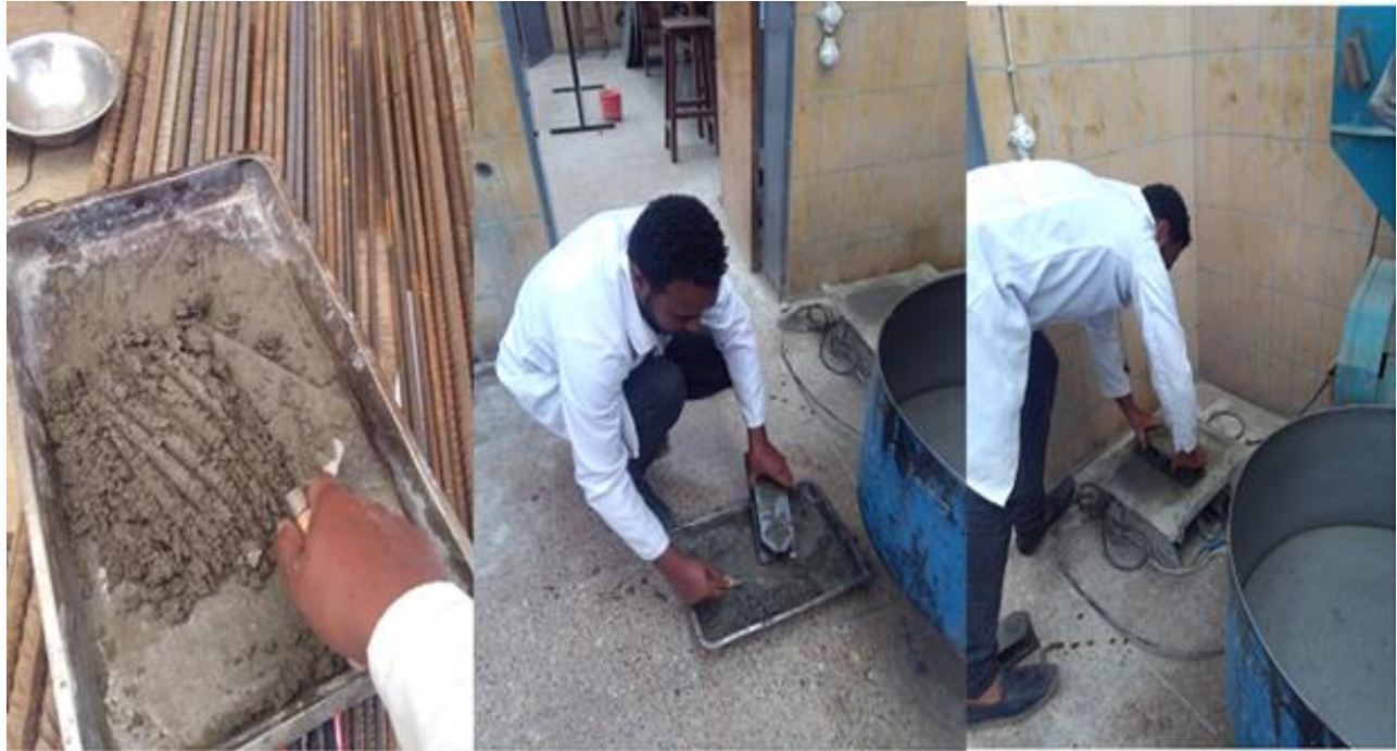
I-9: Mixing, molding and vibrating mortar cubes
