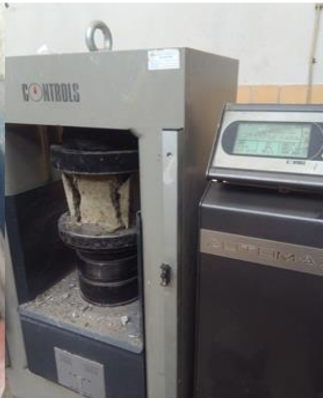
I-13: Concrete under curing and compressive strength test
