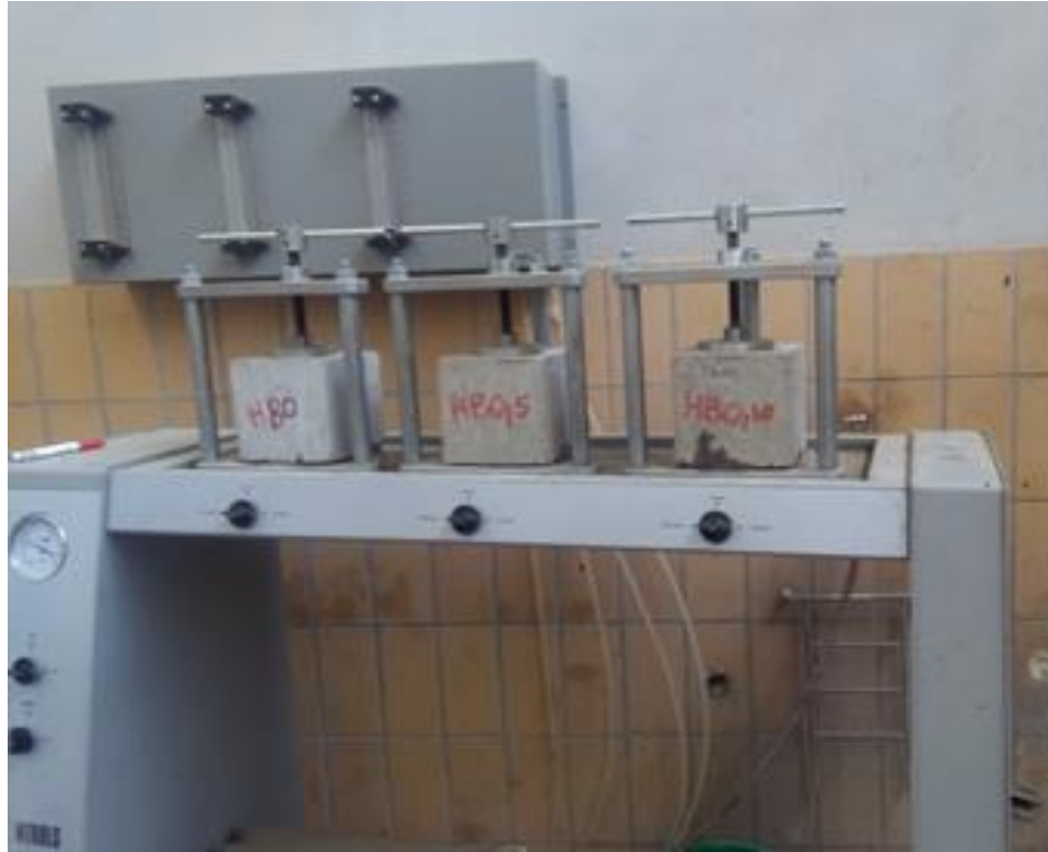
I-14: Concrete cubes assembled on Permeability apparatus
