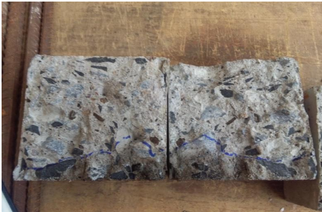
I-15: Concrete sample after splitting at the end of the water permeability test
