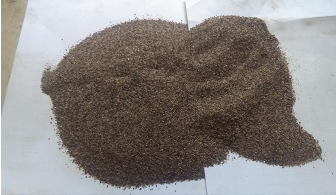
Figure 3-3 Sand prepared and used for determination of cement strength
