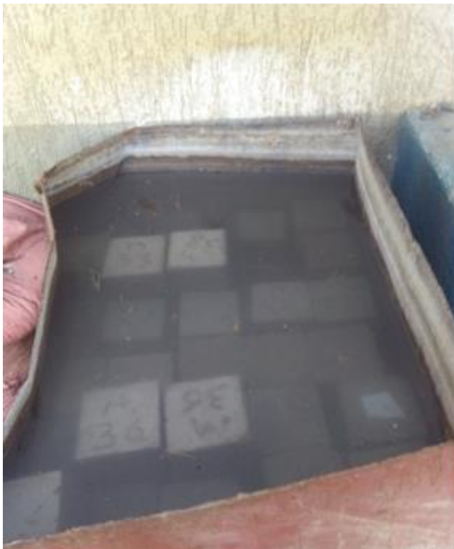
I-13: Concrete under curing and compressive strength test
