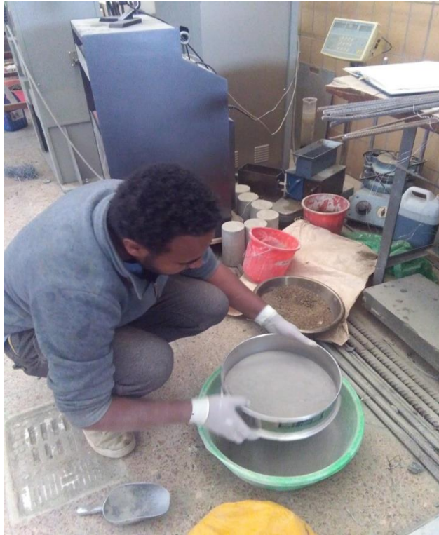
I-6: Sieving crusher dust through 150 \mu sieve
