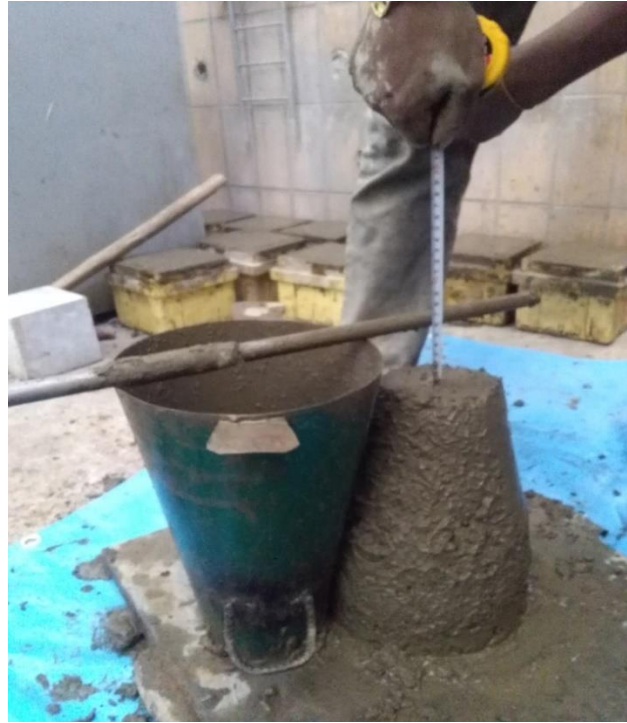
I-12: slump test
