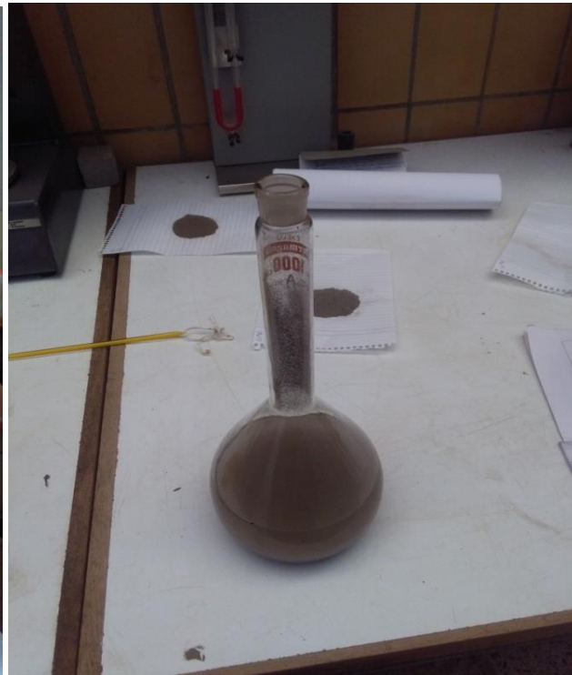
I-5: Pycnometer used for determining specific gravity of crusher dust
