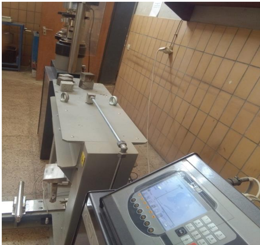
I-10: Measuring compressive strength of mortar cubes
