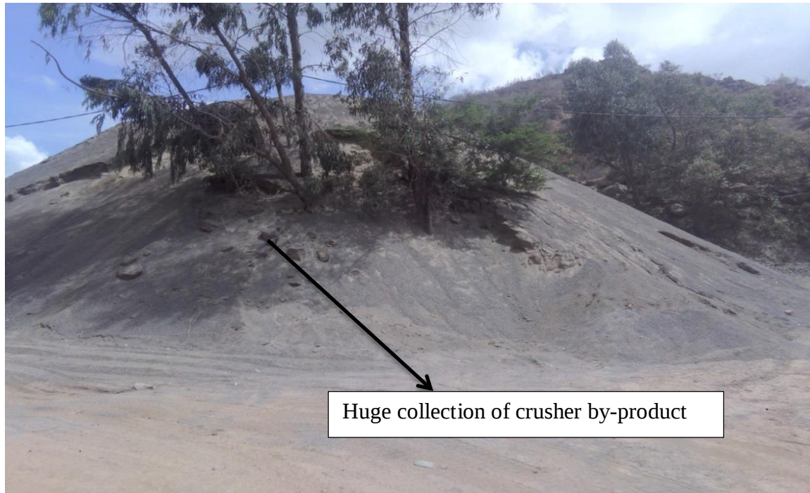
Figure 6-3 Collection of crusher by-product tightening working and storage area (Aggregate production site found in Addis Ababa Akaki Kaliti sub city)
