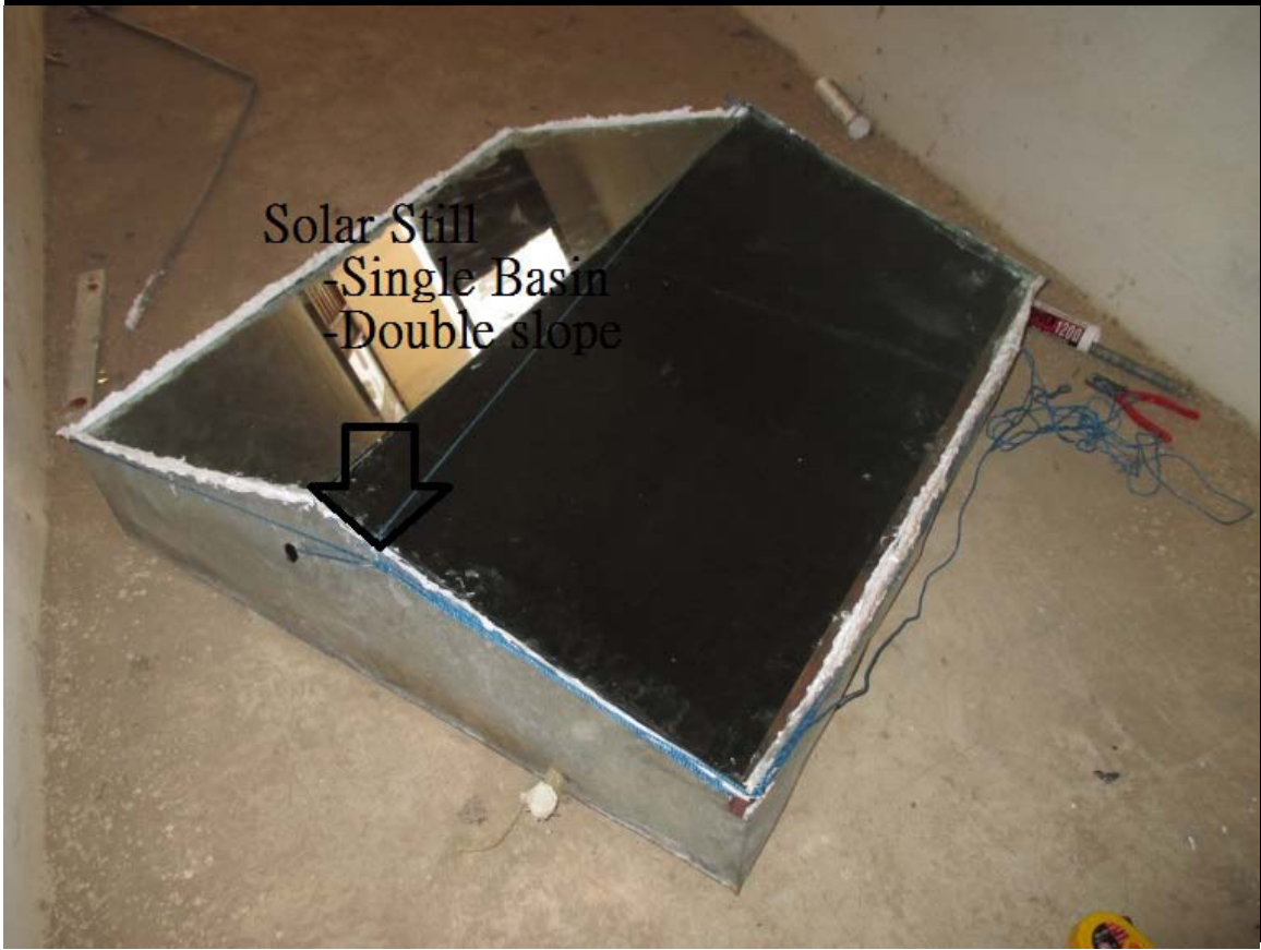
Fig: 3.3 Manufactured single basin double slope solar still
