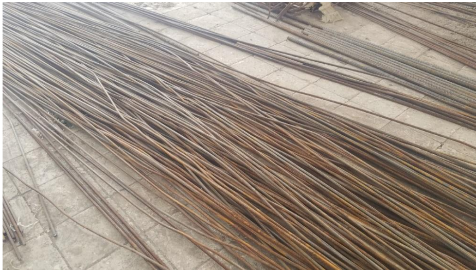
Note. Corroded and zigzagged rebars
