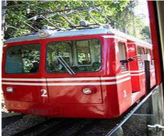
Figure 2.1: Three Phase pantograph on a Corcovado Rack Railway train in Brazil [1]
