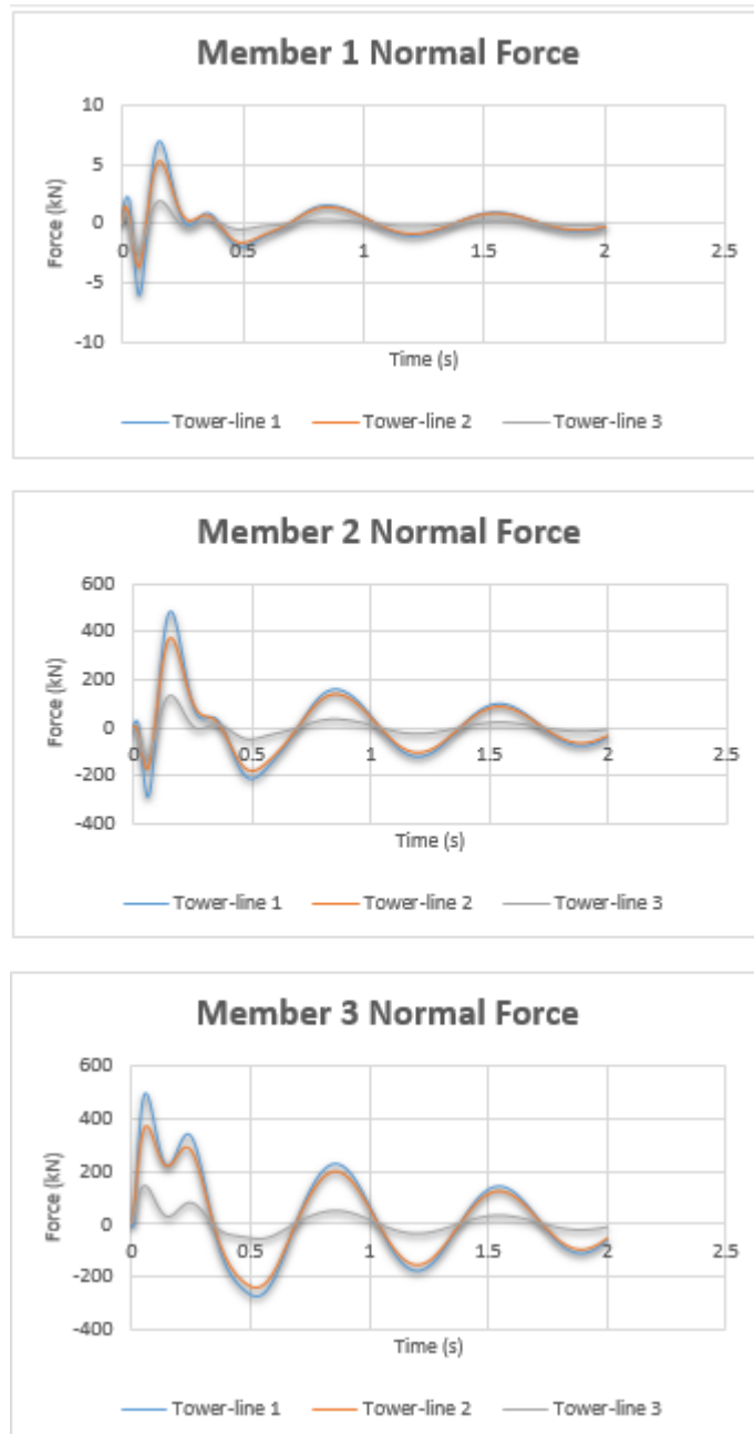
Figure 4-10 Member force response of a tower-line system with identical blast weight and varying standoff distance. Tower-line 1) 3kg and 10m, Tower-line 2) 3kg and 20m, Tower-line 3) 3kg and 50m
