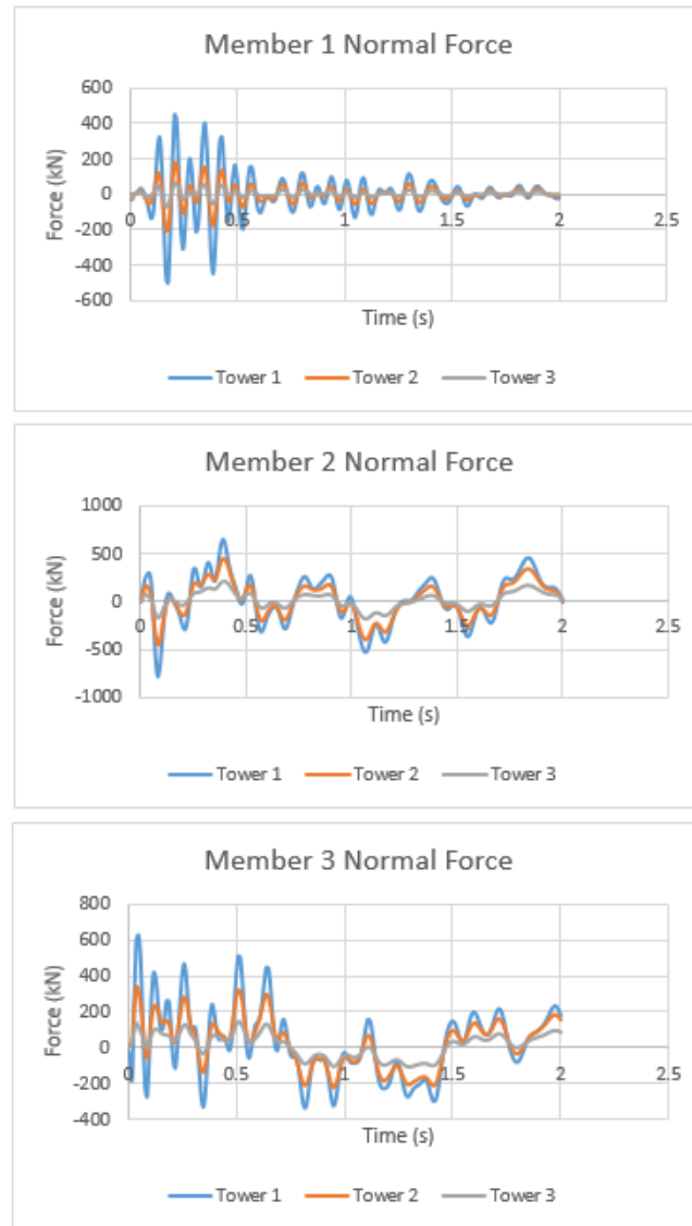
Figure 4-7 Member force response of towers with identical blast weight and varying standoff distance. Tower 1) 3kg and 10m, Tower 2) 3kg and 20m, Tower 3) 3kg and 50m.
