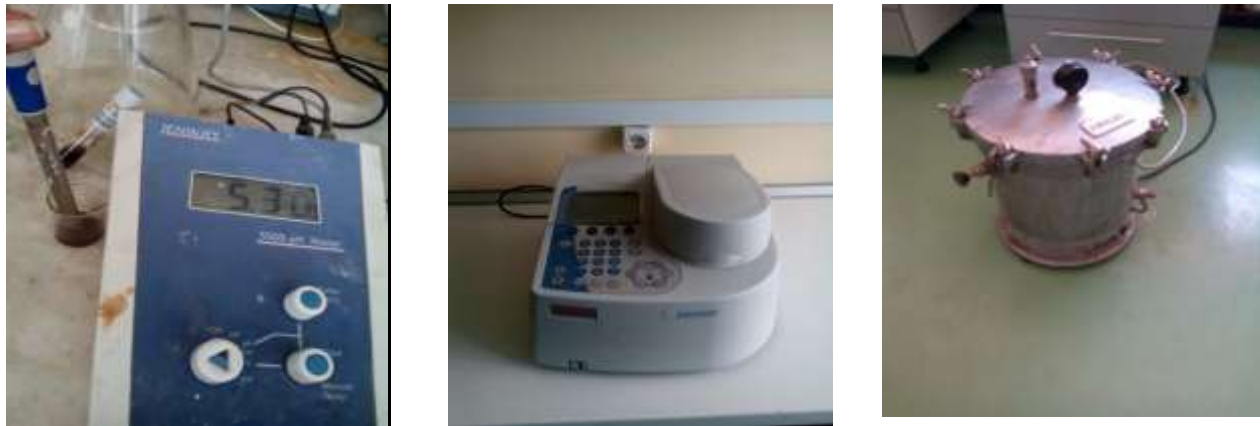
Figure: E5. PH meter, spectrophotometer and 121 °C autoclave respectively
