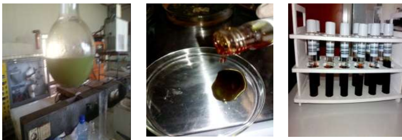
Figure: E3. Etracted pumpkin seed oil with ethanol in 500ml bottel , Extracted pumpkin seed oil on petri dish and extracted oil on using different parameter respectively
