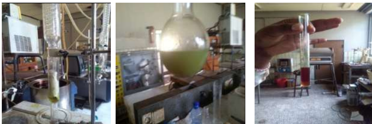
Figure: 3.3. Soxhlet extraction set up, ethanol and oil from soxhlet and extracted oil respectively
