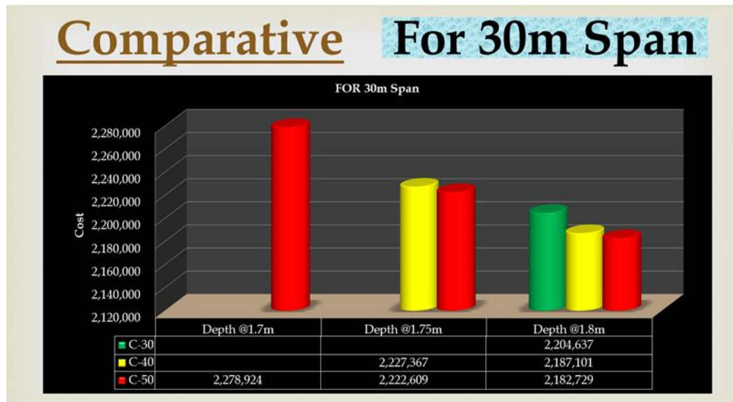
Figure 4-1: Cost comparison chart for 30m span length
