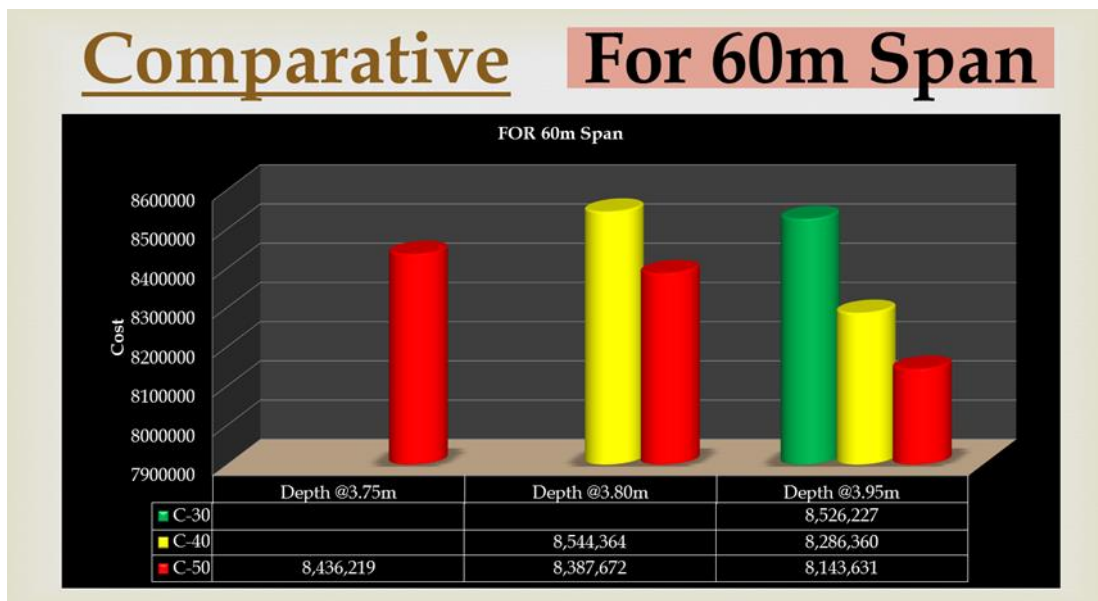
Figure 4-4: Cost comparison chart for 60m span length
