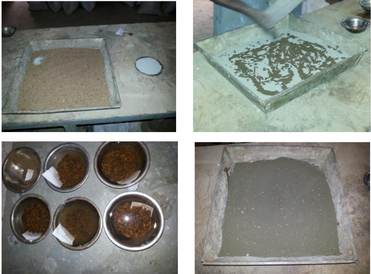
Figure 4.4 Preparation of soil-cement mixture
