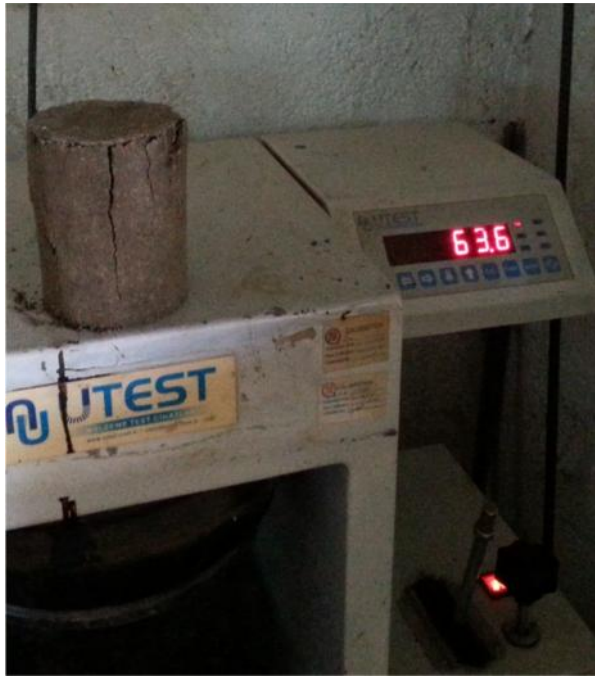
Figure 4.6 Unconfined Compression Test and Test Specimen Preparation
