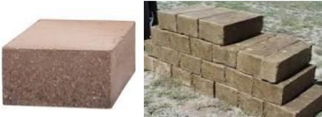
Fig.2.10. Typical compressed earth block [1]
