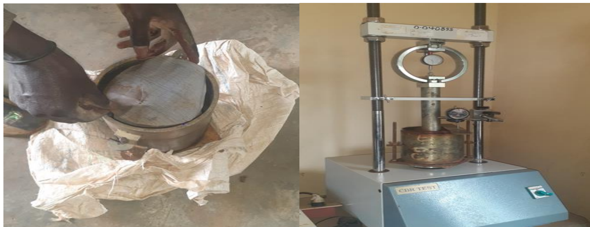
Fig. 4. 15 Conducting CBR test
