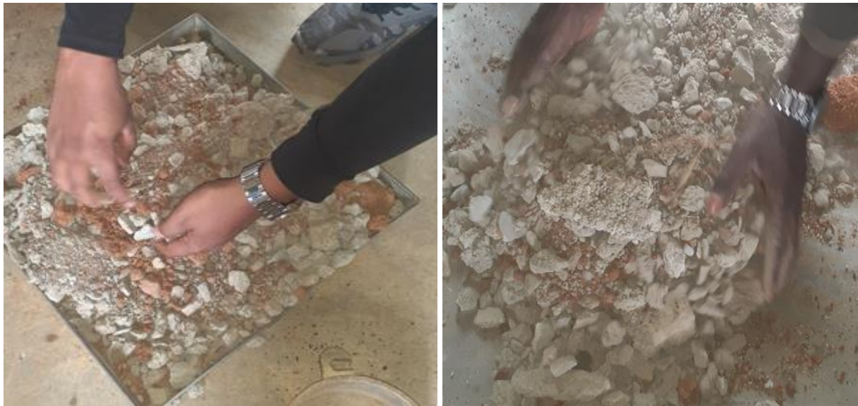
Fig. 3. 5 Mixing CDWs with Clay material
