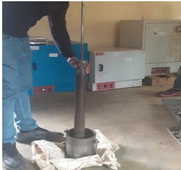
Fig. 4. 9 Procter Compaction test conducting
