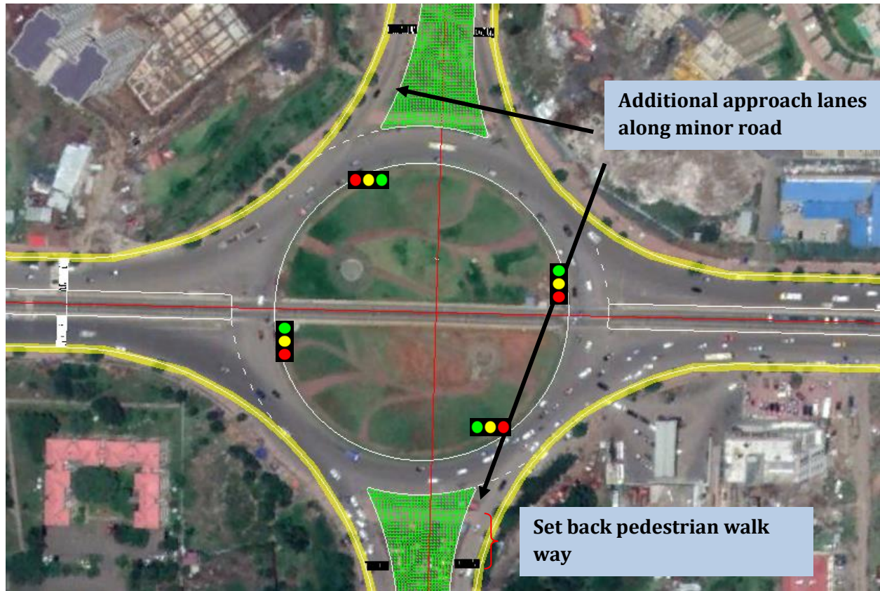
Figure 43 Modified Geometry of CMC Signalized roundabout
