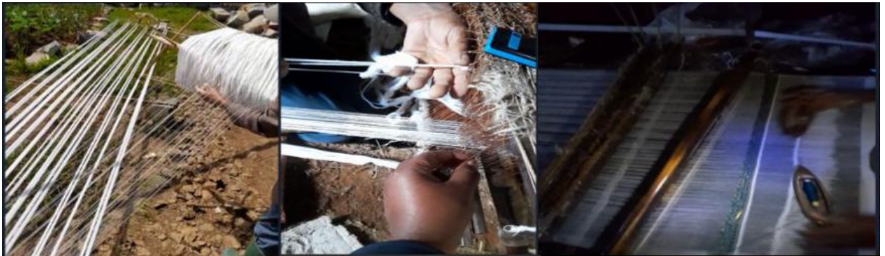
Figure 4.20 Warping and tying threads on looms ( manii ) and design making
