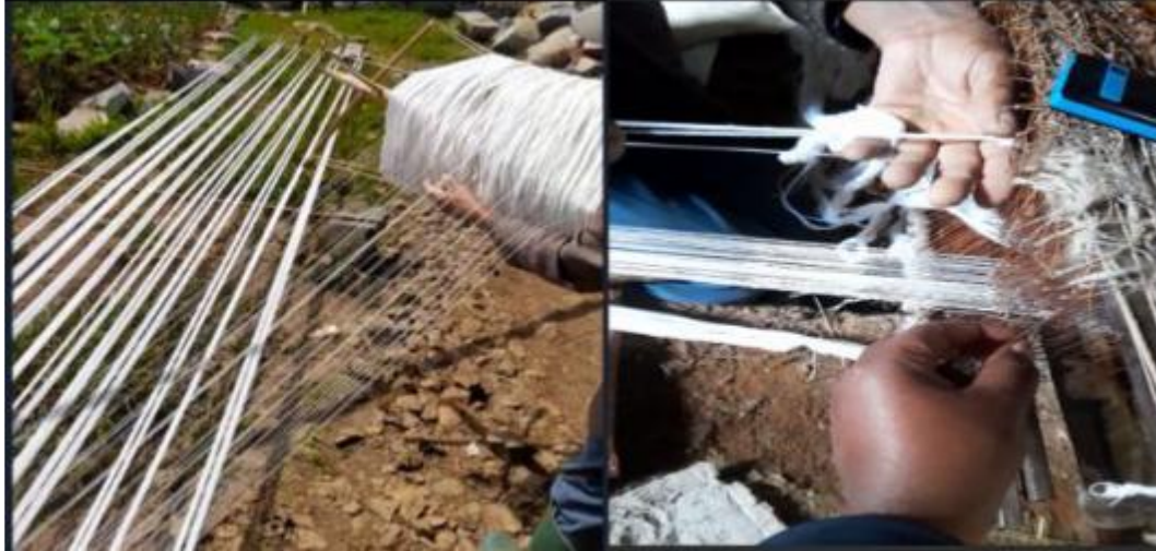
Figure 4.21 Counting performed during warping and tying warps on looms
