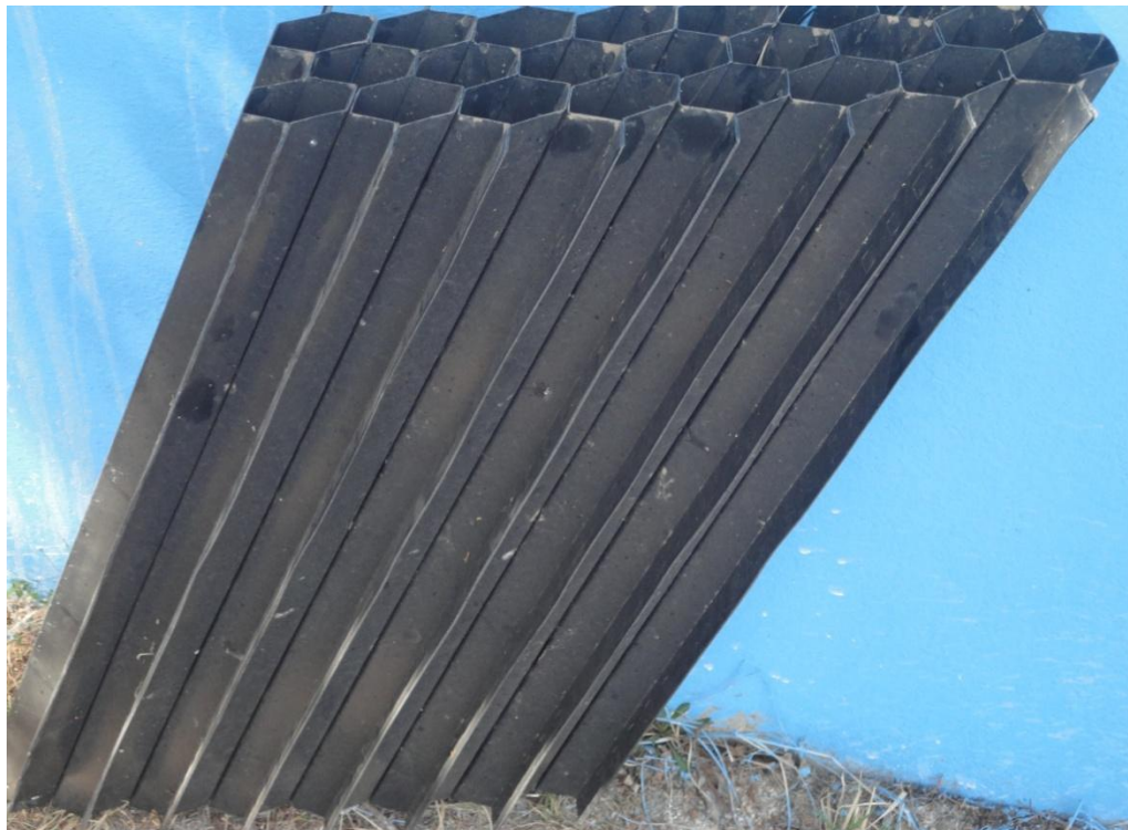
Figure 3-4: The hexagonal types of high rate tube settler (the one used for Legadadi and pilot)
