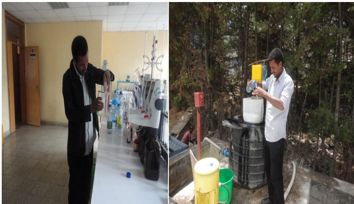
Figure 3-10: Photo's Preparation and addition of coagulant and coagulant aid to the system
