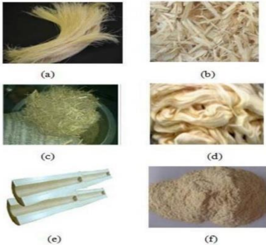
Figure 11: Forms of bamboo being used as composite reinforcement (a) long fibers (b) flake (c) short fibers (d) sliver (e) strips and (f) powder. [21].
