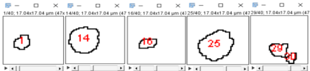
Figure 4.20 Labeled antibubbles under three cycles of ultrasound pulse of amplitude 5V (PNP of 1 MPa).
