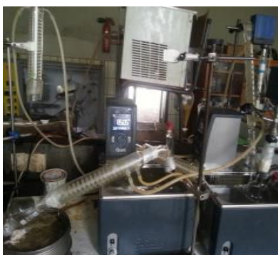
D8: Simple distillation set up
