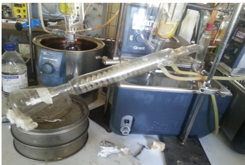
Fig. 4.24 Simple distillation setup to recovery ethanol from water-ethanol mixture
