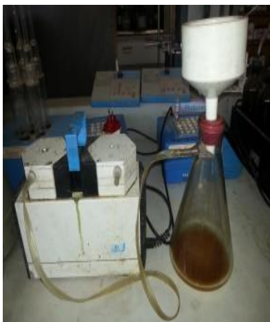
D2: Vacuum filtration unit
