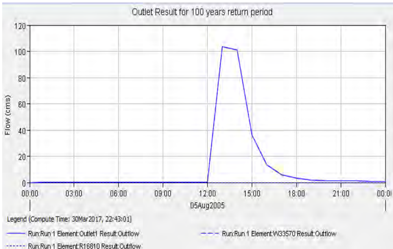
Figure 0-8 HEC- HMS Frequency Hydrograph For 100 years Return Period
