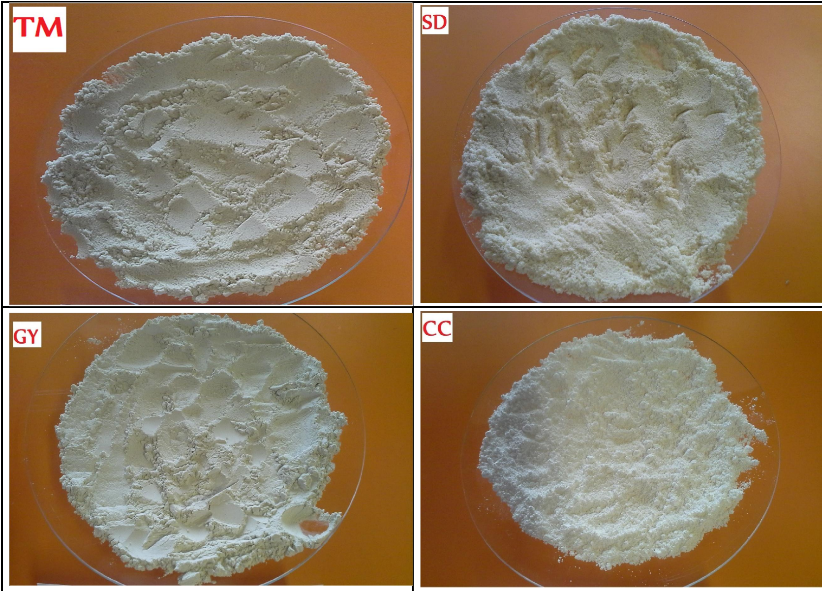
Figure 6: Appearance - Magna teff flour -TQ, Sawdust -SD, Calcium Carbonate -CC and Gypsum -GY
