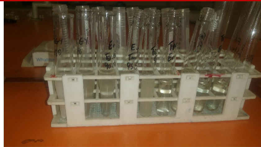
Appendix 6: Precipitation of insoluble salt of calcium using barium solution
