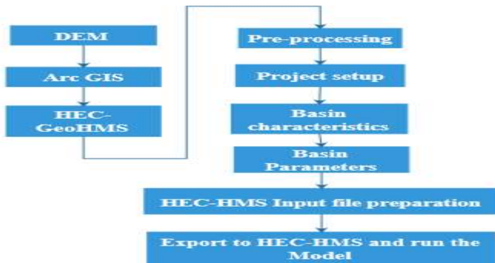
Figure 3-10: HEC-GeoHMS Preprocessing workflow diagram
