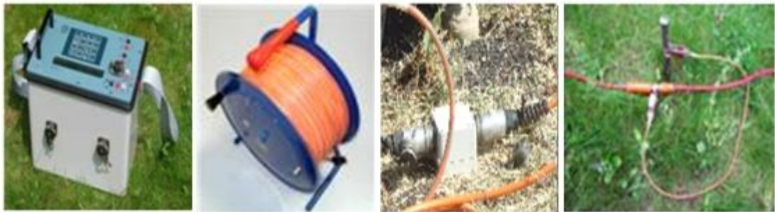
Figure 4.1 Instrumentation of 2D electrical imaging.
