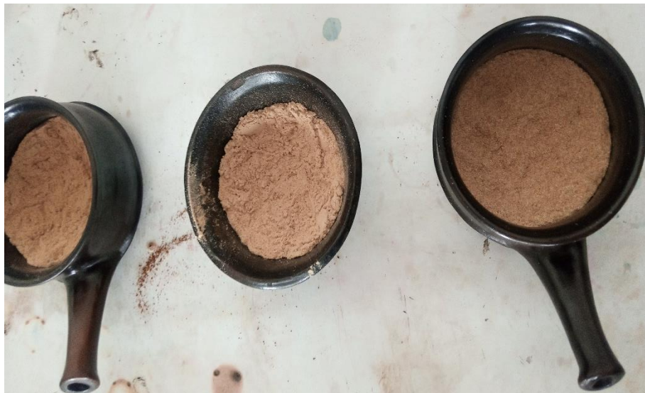
Figure 6: Pulverized Raw Materials Prepared for Carbonization
