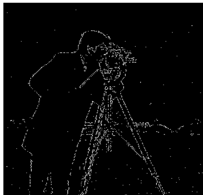
"Sobel" with Hard Thresholding "Gaussian" PSNR = 16.2176
