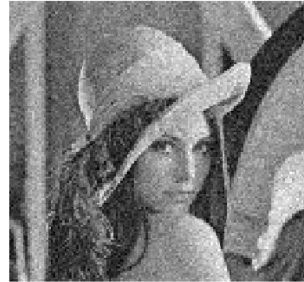
db1 Bayes thresholding with PSNR = 23.3885
