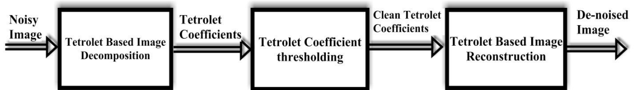
Figure 3.2: Basic steps in Tetrolet based image de-noising step.
