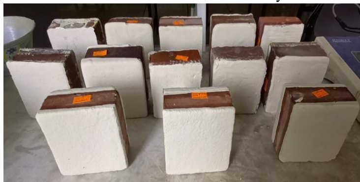
Capping of the bricks with gypsum
