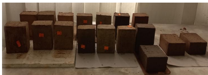
Air drying of the green bricks in the laboratory
