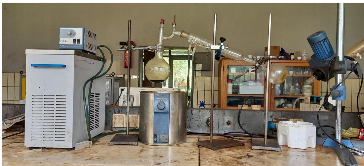
Digestion process of tannery sludge and bottom ash
