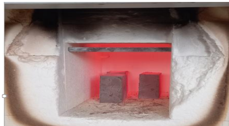
Firing of green bricks
