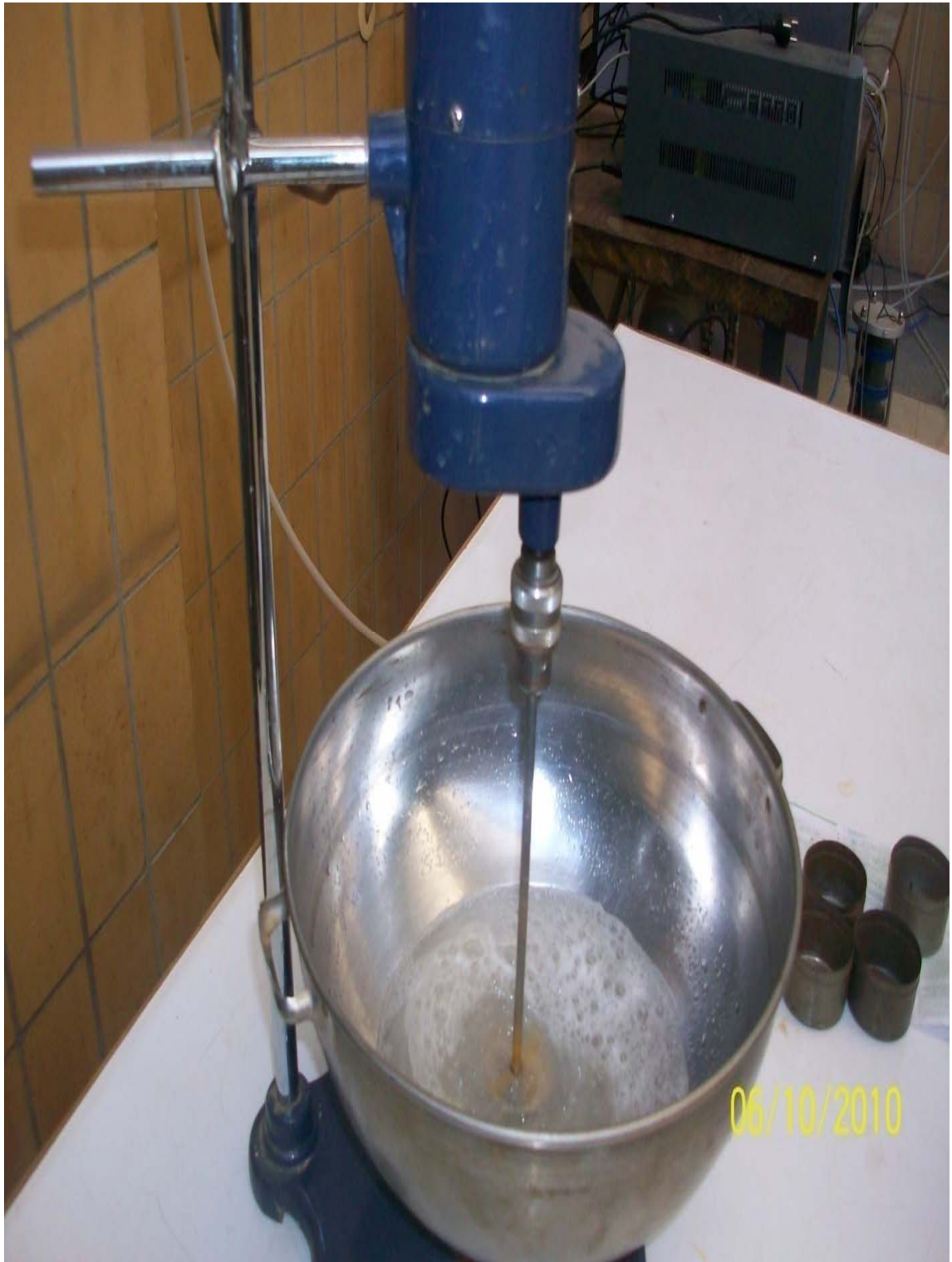
Fig 4.5, water and con-Aid mixing in the mixer
