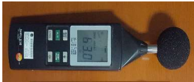
Figure 3. 5 Digital Sound Level Meter (SLM- 816).
