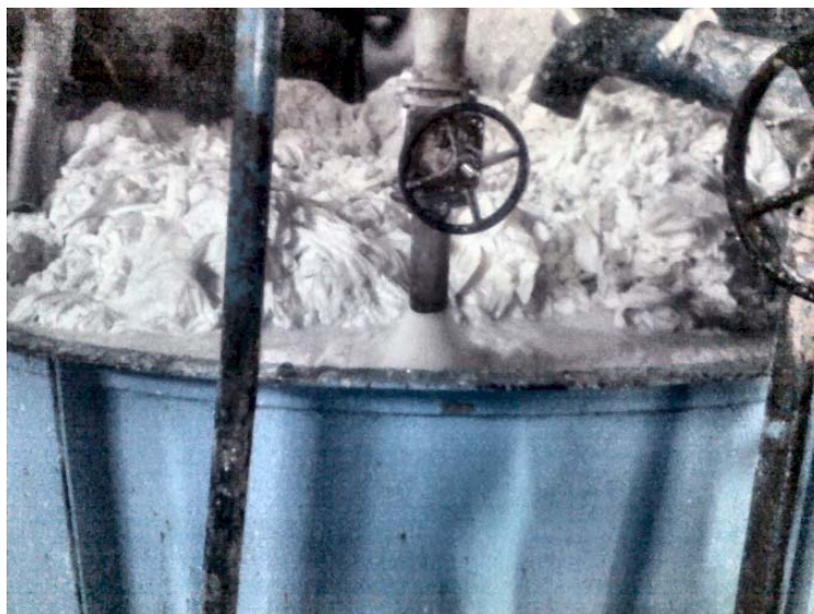
Fig.7 Pulp and paper being disintegrated in the hydropulper
