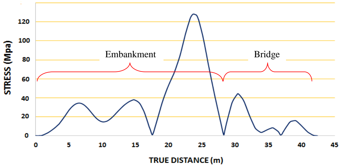
Figure 4.2 stress (MPa) variation along the length (m) of the track (when the wheel moves from bridge to embankment) for speed of 200km/hr
