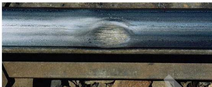
Figure 2.20 General appearance of Wheel Burns (Australian Rail Track Co., (2006))
