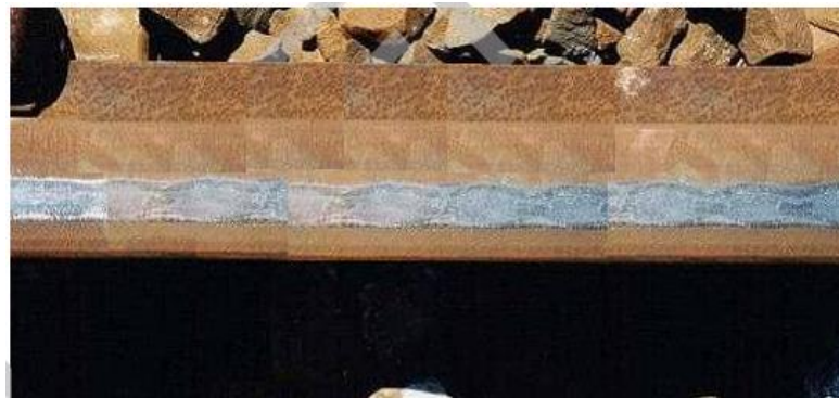
Figure 2.11 short pitch corrugations on the running surface (U.S.DOT, 1984)
