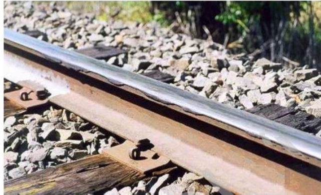
Figure 2.13 Rail plastic flow associated with long pitch corrugations (U.S.DOT, 1984)
