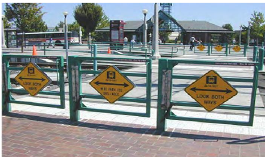
Figure 2-15: Manual swing gate (Source; Korve et al., 2007)
