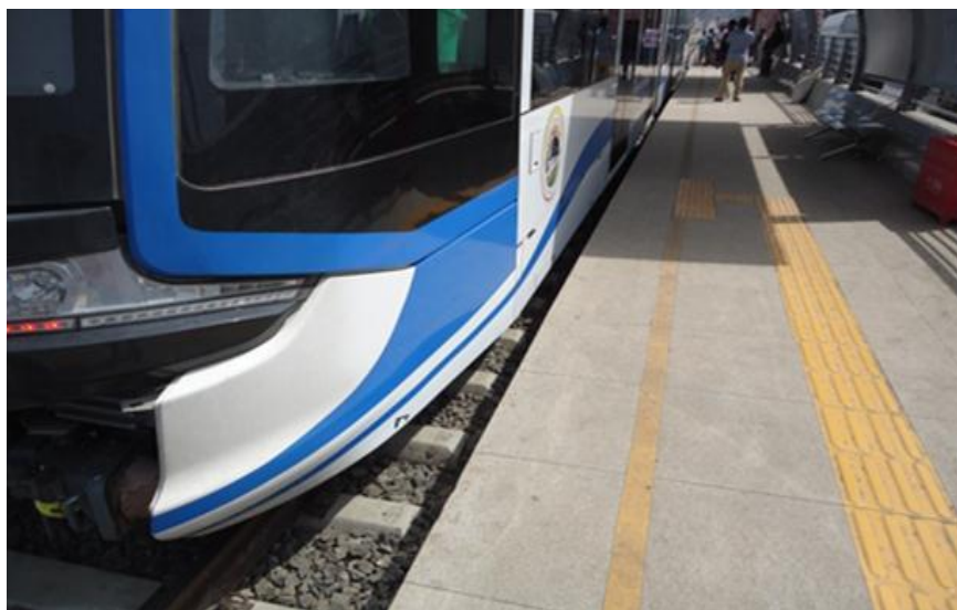
Figure 4-4: Space between the train and the platform edge at AALRT
