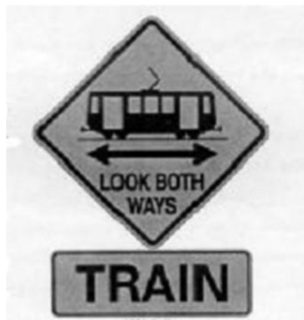
Figure 2-12: Light rail transit crossing signs
