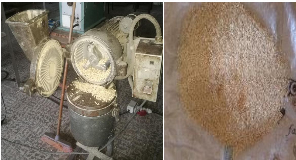
Figure 3.5: Attrition mill and corn cob after grinding
