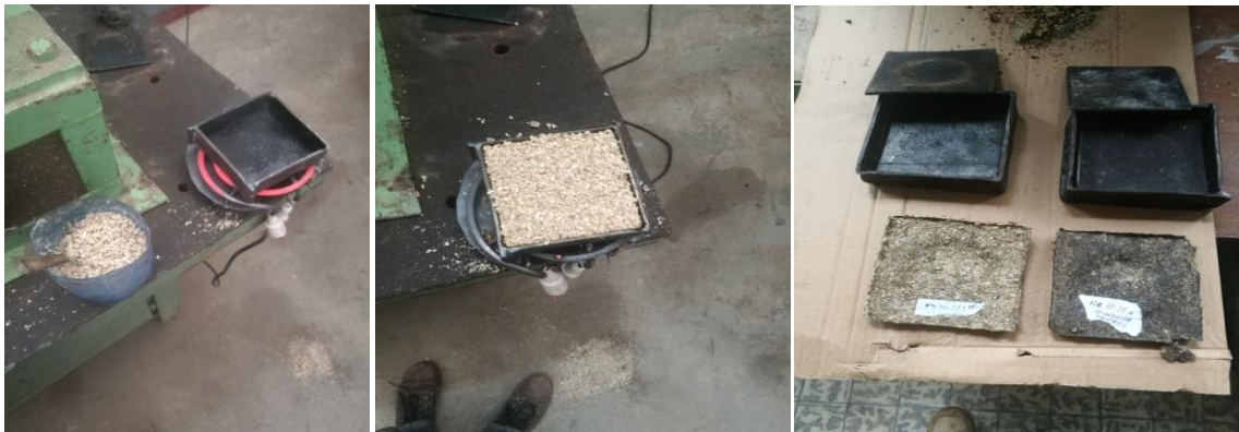
Figure 3.7: Metallic mould and plates
