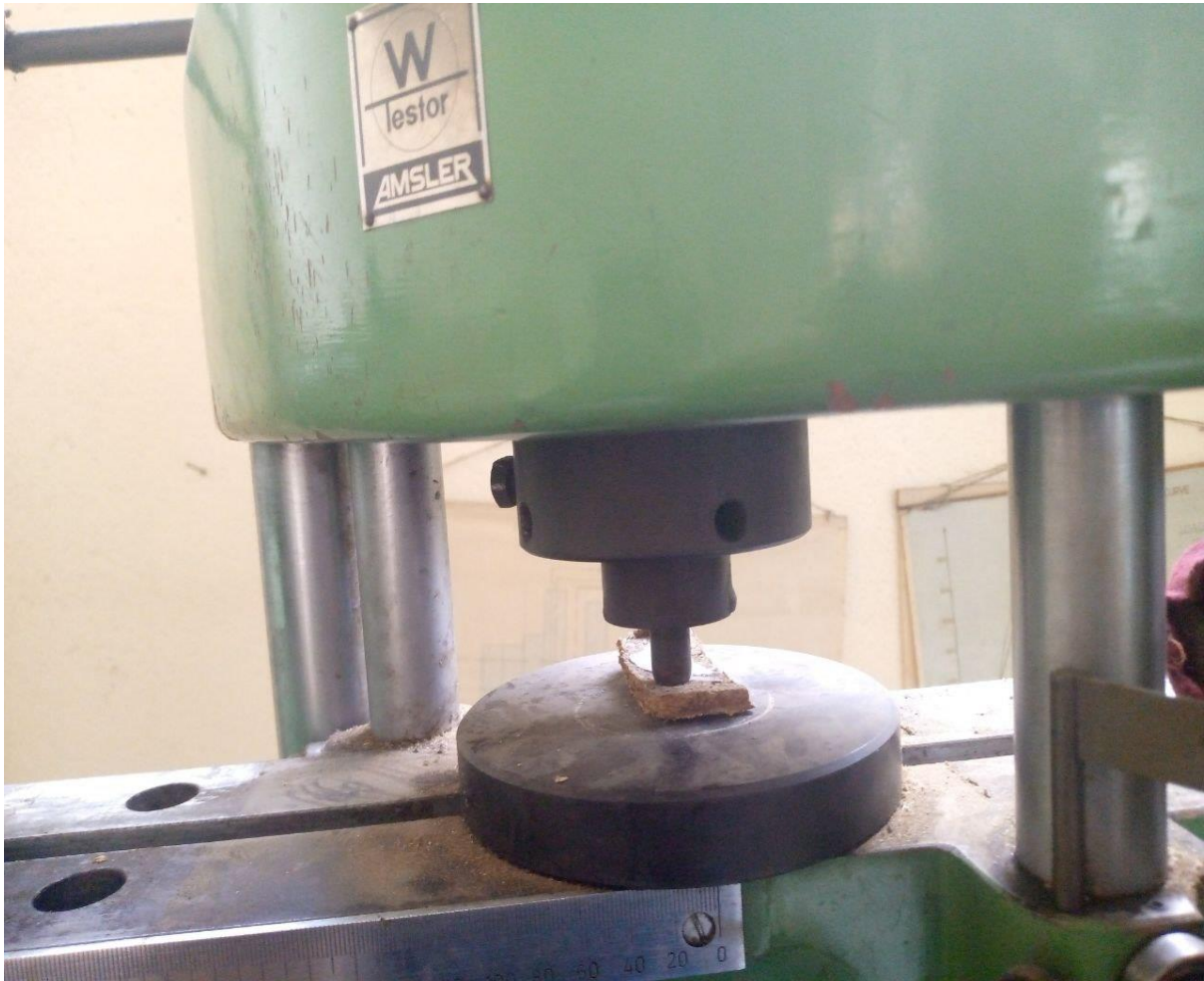
Figure 4.2: Hardness measuring setup of particle board (ASTM Roell, M.FOS.013, and ASTM D1037-06a).
