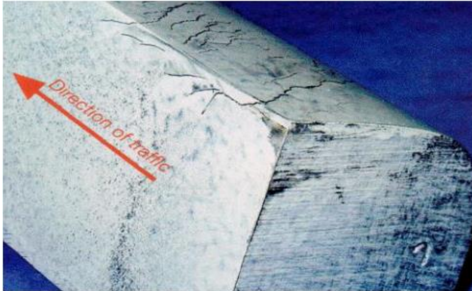
Figure 2: Rolling Contact Fatigue crack growth [18]
